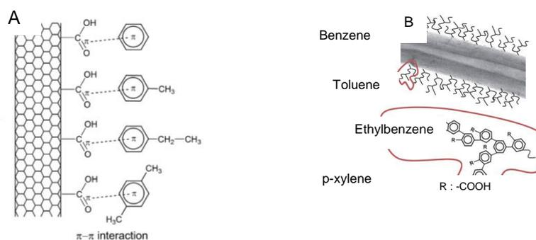
**Figure 1:** (A)  $\pi$ - $\pi$  stacking interactions between carboxylic groups and BTEX<sup>5</sup>, (B) Poly(phenylene) derivative grafted onto CNTs.
