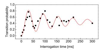
Fig. 3. Experimental observation of the Rabi oscillations for  $B=1.68\,\mathrm{mT}$  at maximum intensity  $I_0\simeq 6\,\mathrm{W/cm^2}$ . The line is a fit corresponding to classical Rabi oscillations attenuated by an exponential decay. The frequency of the oscillations is  $16(1)\,\mathrm{Hz}$ , the time constant of the decay is about  $100\,\mathrm{ms}$  which corresponds to the coherence time of the interrogation laser.
