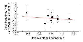
Fig. 4. Clock frequency vs atomic density. All the points have been corrected for the Zeeman and the light shifts. The line is a linear fit to the data. We have  $n_0 = 2.5 \times 10^{11} \, \mathrm{at/cm^3}$ .
