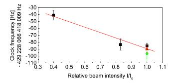
Fig. 2. Light shift due to the interrogation laser for different values of the magnetic field.  $\blacksquare$ : 1.68 mT,  $\blacktriangle$ : 1.4 mT,  $\bigstar$ : 1.12 mT.  $I_0 \simeq 6 \, \text{W/cm}^2$  corresponds to the clock laser intensity at standard operating conditions. The line is a linear fit to the data.
