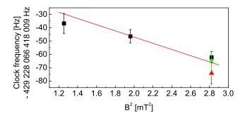
Fig. 1. Dependence of the clock frequency on the static magnetic field. The line is a fit to the experimental data with an adjustable offset, the slope being fixed to the theoretical value of Ref. <sup>20</sup>  $\blacksquare$ :  $I/I_0 = 1$ ,  $\blacktriangle$ :  $I/I_0 = 0.83$ ,  $\bigstar$ :  $I/I_0 = 0.4$ .
