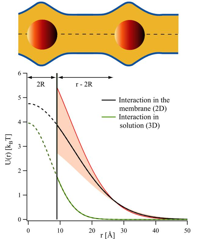
FIG. 3: Interaction potential  $U(r)$  of the BuSn12 particles within the bilayers, obtained by taking the inverse Fourier transform of the solid line and the shaded area in Figure 2 (see text for the numerical values). The lower curve is the interaction potential of the particles in ethanol. The solid vertical line marks the hard core interaction with radius  $4.5 \text{\AA}$
