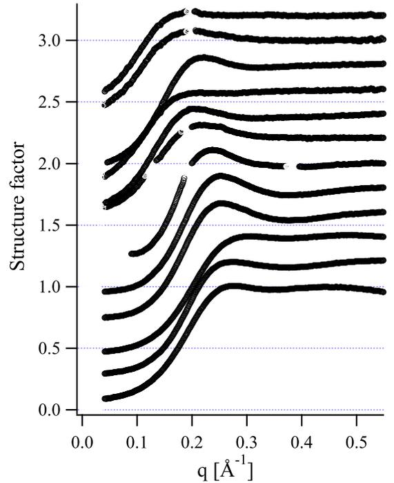
FIG. 1: Structure factors  $S(q)$  of the 2D fluid formed by the BuSn12 particles in the plane of the membranes, for different concentrations, from top to bottom:  $n = 0.217, 0.231, 0.429, 0.434, 0.451, 0.584, 0.801, 1.102, 1.275, 1.976, 2.147,$  and  $2.304 \cdot 10^{-3}\text{\AA}^{-2}$ . The curves are shifted vertically in steps of  $0.2$ . Gaps in the curves correspond to the presence of (weak) lamellar peaks, due to occasional alignment defects, mainly taking the form of oily streaks.
