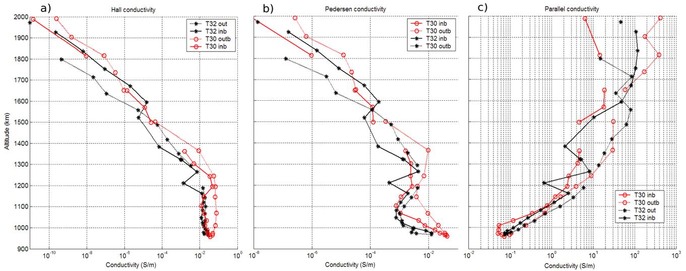
**Fig. 6.** Electrical conductivities (S/m) as a function of altitude (km) during the inbound (continuous lines) and outbound (dotted) of the T30 (red) and T32 (black) flybys: Hall (a), Pedersen (b) and parallel conductivities (c).
