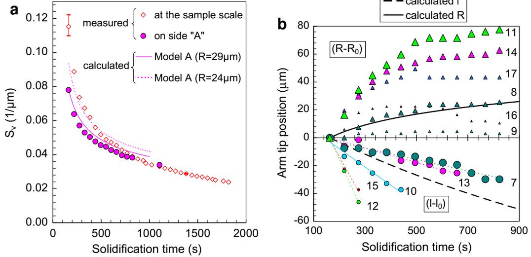
Fig. 11. Variation with time of (a) the measured and computed specific solid-liquid interface area,  $S_v$ , for the dendrite arms that follow model A and (b) the dimensions of these arms.
