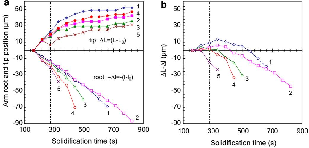
Fig. 10. Variation with time of (a) the relative positions of the dendrite arms tips ( $\Delta L$ ) and roots ( $\Delta l$ ) that follow model B (to facilitate comparison with tips, the positions of the roots are plotted along a negative  $y$ -axis even though  $l$  increases) and (b) the difference ( $\Delta L - \Delta l$ ) between growth of the tips and filling of the roots.
