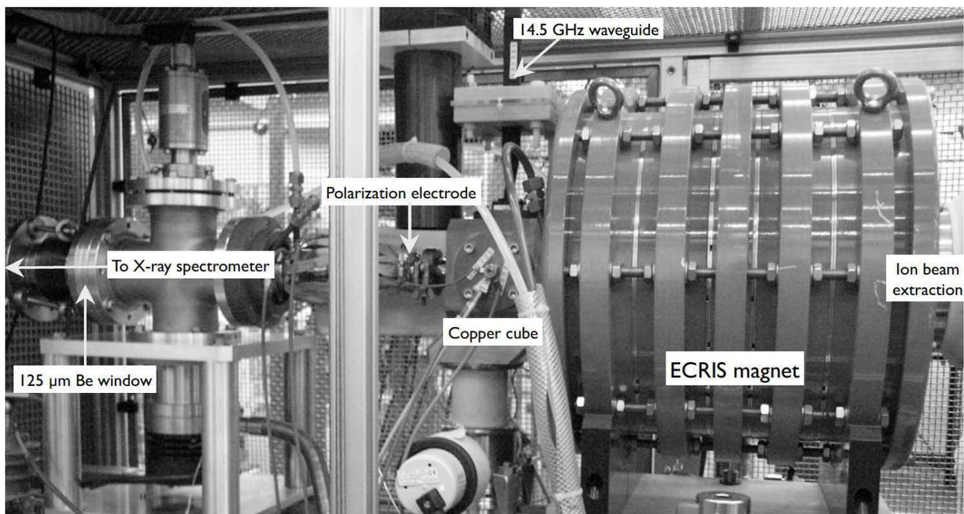
Figure 3: The SIMPA ECRIS and its connection to the spectrometer
