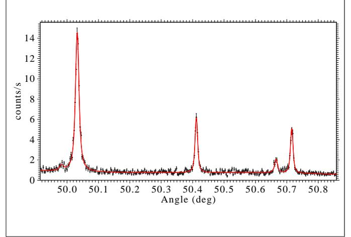
Figure 22: (color online) Experimental survey dispersive spectrum. Left peak:  $1s^2 2s^2 2p^1 P_1 \rightarrow 1s^2 2s^2^1 S_0$  in  $\text{Ar}^{14+}$ , central peak:  $1s 2s^3 S_1 \rightarrow 1s^2^1 S_0$  in  $\text{Ar}^{16+}$ , right peaks:  $1s 2s 2p^2 P_{1/2,3/2} \rightarrow 1s^2 2s^2 S_{1/2}$  in  $\text{Ar}^{15+}$ . The line represents a fit using a sum of Voigt profiles.
