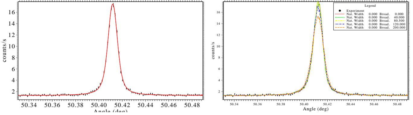
Figure 14: (Color online) Voigt profile (left) and simulated profiles with different line widths (right) fitted to an experimental dispersive mode spectrum. The Voigt profile fit yield a  $\chi^2 = 1.42$  and the optimum simulated profile one (for a Gaussian broadening of 80 meV) gives a  $\chi^2 = 1.26$ . The difference in angle between the peak position between the two fits is equal to  $1.86(7) \times 10^{-3}$  degrees.
