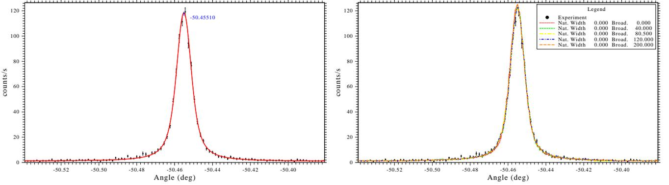
Figure 13: (Color online) Voigt profile (left) and simulated profiles with different line width (right) fitted to an experimental non-dispersive mode spectrum. The Voigt profile fit yield a  $\chi^2 = 1.12$  while the simulated ones gives  $\chi^2$  ranging from 1.2 to 1.4 (the variation is mostly due to the statistic of the simulated profiles). The difference in angle is equal to  $1.3 \times 10^{-4}$  degrees.
