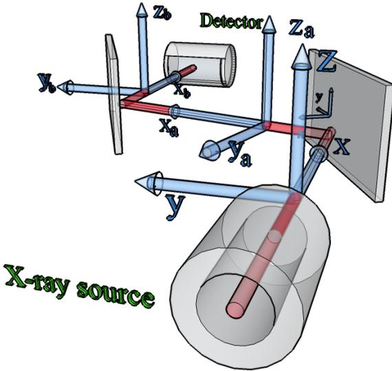
Figure 11: (Color online) Geometry of the DCS in a non-dispersive setup with the central line and the tri-orthogonal  $xyz$  axis along the central line.
