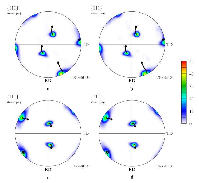
**Fig. 13.** Influence of remeshing on the crystal rotation of single grains, during a plane strain compression of  $\varepsilon = 1$ . (a, b) and (c, d) represent two different grains of the polycrystal of Fig. 12. (a, c) Infrequent remeshing (every 0.4 strain), (b, d) frequent remeshing (every 0.1 strain). The dots represent the initial orientation, the thick line its trajectory with strain, and the colour density plots the final orientation spreads.
