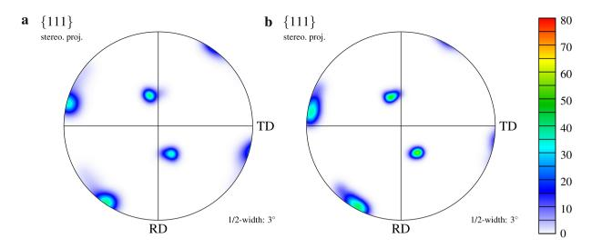
Fig. 19. Examples of (a) experimental and (b) finite element in-grain orientation spreads at  $\varepsilon$  = 1.2, for two grains of approximately the same average orientation.
