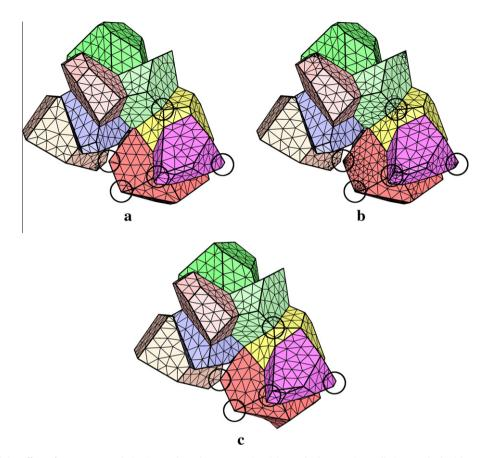
**Fig. 8.** An illustration of the effect of geometry regularization and meshing properties. (a) Standard Voronoi tessellation meshed with  $p_l \rightarrow \infty$ , (b) standard Voronoi tessellation with  $p_l = 1.5$ , (c) regularized Voronoi tessellation with  $p_l = 1.5$ . The zones of interest are marked with circles. Note the poor-quality elements in (a) and the mesh overrefinements in (b) near the small edges; (c) shows high-quality elements and no mesh overrefinements.
