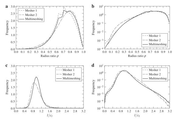
**Fig. 11.** Influence of the multimeshing strategy on mesh quality. Distributions of the (a-b) element qualities and (c-d) relative element sizes, in linear and logarithmic scales. Mesher 1 is the Netgen mesher + the Gmsh optimization; mesher 2 is the Netgen mesher + both the Netgen and Gmsh optimizations. Data collected on  $10^5$  grains.
