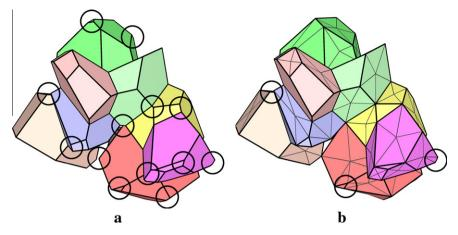
Fig. 4. Voronoi tessellation regularization: (a) original Voronoi tessellation and (b) equivalent regularized Voronoi tessellation. The small edges are surrounded and the face interpolations triangles are marked in gray. Case of a 9-grain polycrystal.
