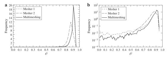
**Fig. 10.** Influence of the multimeshing strategy on mesh quality. Distributions of O in (a) linear and (b) logarithmic scales. Mesher 1 is the Netgen mesher + the Gmsh optimization; mesher 2 is the Netgen mesher + both the Netgen and Gmsh optimizations. Data collected on  $10^5$  grains.
