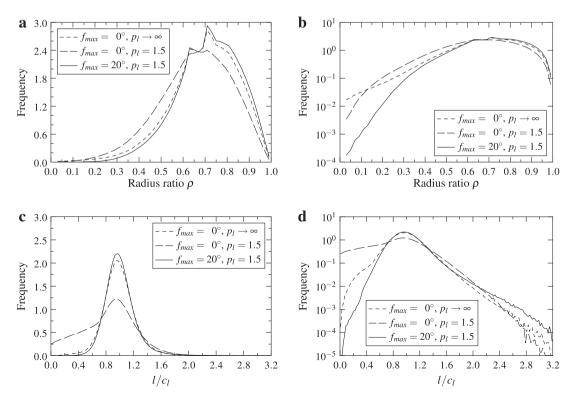
Fig. 9. Mesh quality: (a-b) element qualities and (c-d) relative element sizes for different meshing strategies. Data collected on 10<sup>5</sup> grains.
