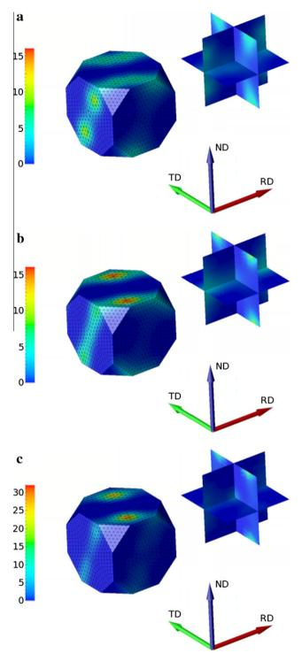
**Fig. 18.** Macrotextures in an aluminium alloy deformed in plane strain compression. (a) Experiments, (b) finite element model, (c) Taylor model. Note the different color scales between (a and b) versus (c). The positions in Rodrigues' space of the  $\beta$ -fiber components are: S = (0.254, -0.235, -0.291), (-0.254, 0.235, 0.291) and (0.254, 0.235, 0.291); Brass = (-0.414, -0.132, 0.318) and (0.414, 0.132, 0.318); Copper = (-0.132, -0.318, 0.414) and (0.132, 0.318, 0.414) [41].
