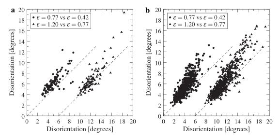
**Fig. 21.** Correlation between the orientation spreads at different strains, in an aluminium polycrystal submitted to plane strain compression. (a) Experiments, (b) finite elements. The right-hand side data clouds have been shifted 6° along the *x*-axis for clarity.
