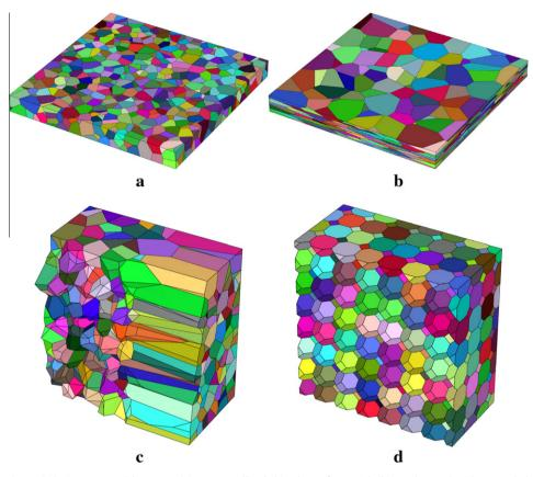
**Fig. 14.** Various polycrystal morphologies generated by Neper. (a) A recrystallized thin sheet of material, (b) a polycrystal with a morphological texture, (c) a mixed columnar/equiaxed grain ensemble representative of solidification microstructures, (d) a set of truncated octahedra. All polycrystals are made of about 1000 grains. (c–d) are cut for the illustration.
