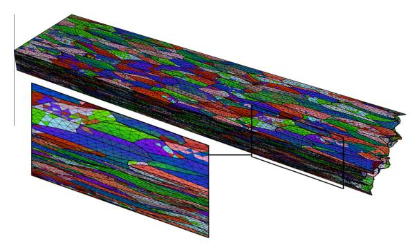
**Fig. 17.** A 3000-grain Voronoi tessellation deformed in plane strain compression to  $\varepsilon = 1.4$  (75% thickness reduction). The mesh contains 973,000 elements and 1,336,000 nodes. The undeformed polycrystal is illustrated in Fig. 1. Color is related to crystal orientation:  $\underline{v}$  being the Rodrigues vector representing the orientation, the RGB color levels are  $255 \times (v_i + \sqrt{2} - 1)/[2 \times (\sqrt{2} - 1)]$ .
