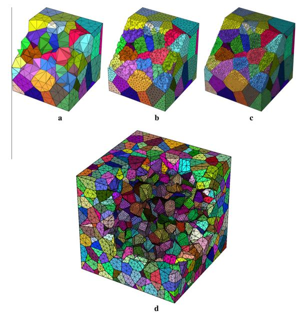
**Fig. 15.** Various levels of mesh refinements. (a–c) Coarse, medium and fine discretization meshes of a 100-grain polycrystal. (d) Heterogeneous mesh refinement of a 2000-grain polycrystal: inner grains with fine meshes and outer grains with coarse meshes.
