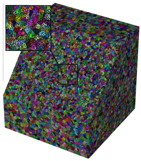
Fig. 16. Free meshing of a 10<sup>5</sup>-grain Voronoi tessellation. The mesh contains 19,600,000 10-node elements and 26,400,000 nodes.
