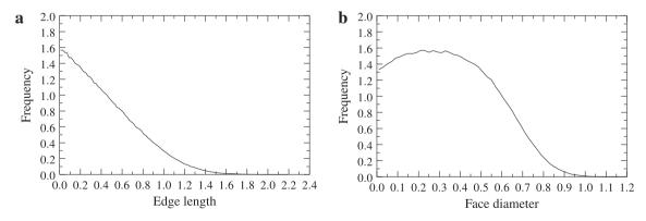
Fig. 3. Particular statistics of Voronoi tessellations. (a) Edge lengths, (b) face diameters. The data are given for grains of unit volume on average. The face diameter is based on the equivalent circle. Note the large number of small entities. Data collected on 10<sup>5</sup> grains.
