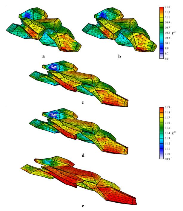
**Fig. 12.** Remeshing with transport of microstructural variables. Case of a plane strain compression of  $\varepsilon$  = 1: (a)  $\varepsilon$  = 0.4, (b)  $\varepsilon$  = 0.4 after remeshing, (c)  $\varepsilon$  = 0.8, (d)  $\varepsilon$  = 0.8 after remeshing, (e)  $\varepsilon$  = 1.0. The element colors are related to the critical resolved shear stress  $g^{\alpha}$ .
