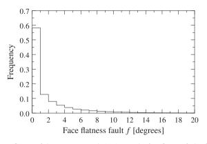
**Fig. 6.** Influence of the geometry regularization on the face flatness faults, for a maximum allowed value of  $f_{max} = 20^{\circ}$ . Note that most of the angles are much smaller. Data collected on  $10^5$  grains (all faces).
