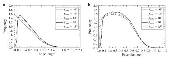
**Fig. 5.** Influence of the geometry regularization on the (a) edge length and (b) face diameter distributions, for increasing values of the maximum allowed flatness faults,  $f_{max}$ . On (a), the dotted line denotes the length under which the edges are considered to be "small" and so are designated for deletion. The data are given for grains of unit volume on average. The face diameter is based on the equivalent circle. Data collected on  $10^5$  grains.
