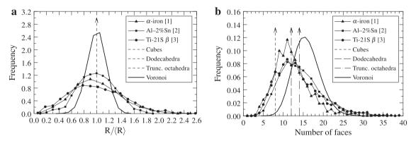
**Fig. 2.** Main statistics of polycrystal morphologies. (a) Distribution of grain size, (b) distribution of the number of grain faces. *R* is the equivalent sphere radius. The arrows denote Dirac-type distributions.
