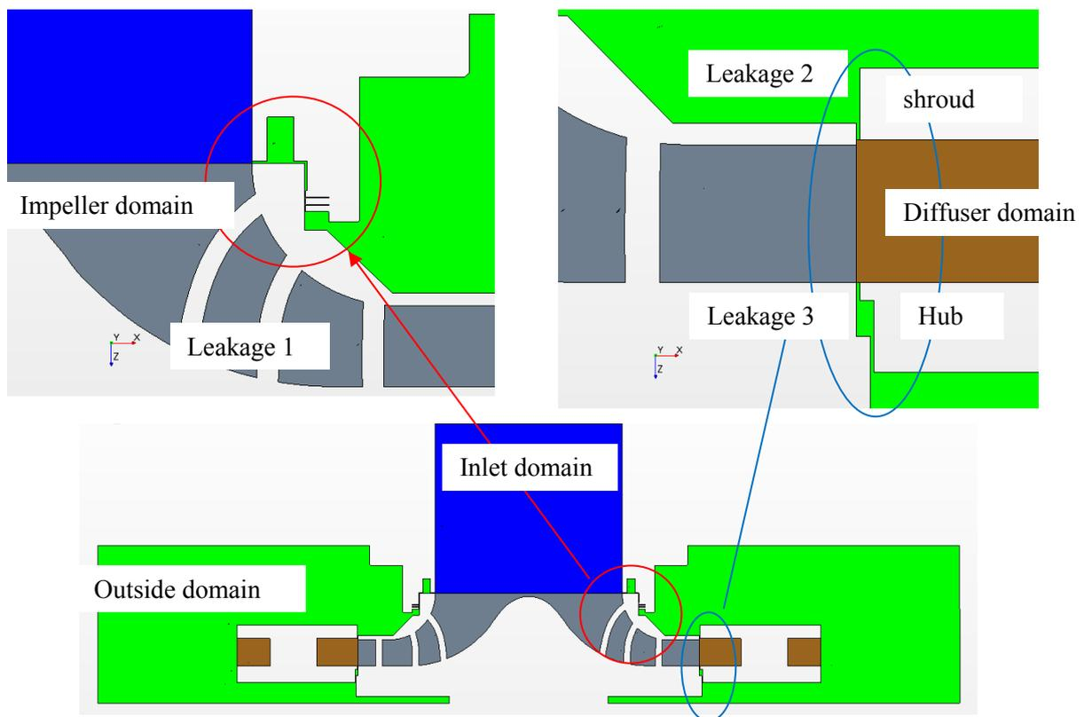
**Figure 6.** Regions modelled. Details of fluid leakages.
