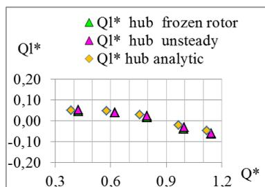
Figure 10. Fluid leakages at impeller/diffuser hub
