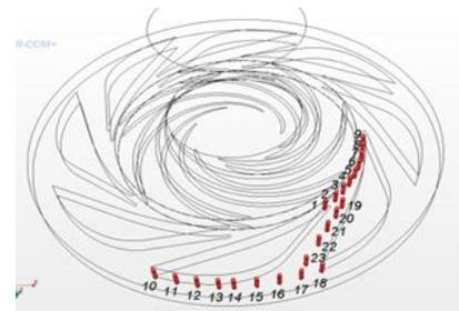
**Figure 3.** Impeller different angular positions relative to the diffuser vanes.
