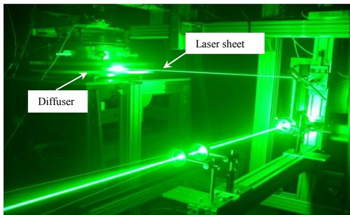
**Figure 1.** Apparatus: PIV measurement, laser sheet.
