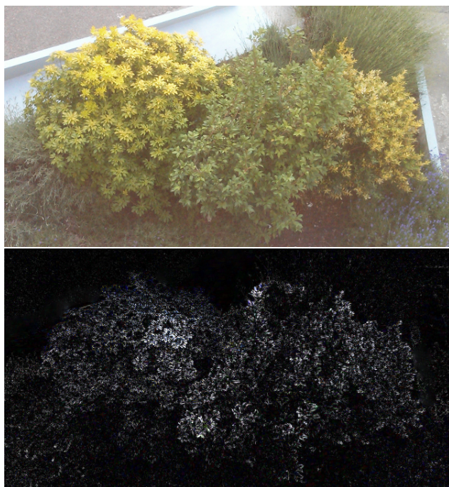
Figure 1: Top: image of small bushes taken from a fixed point of view. Bottom: the brightest areas show the biggest displacement of the vegetation during a period of one second.
