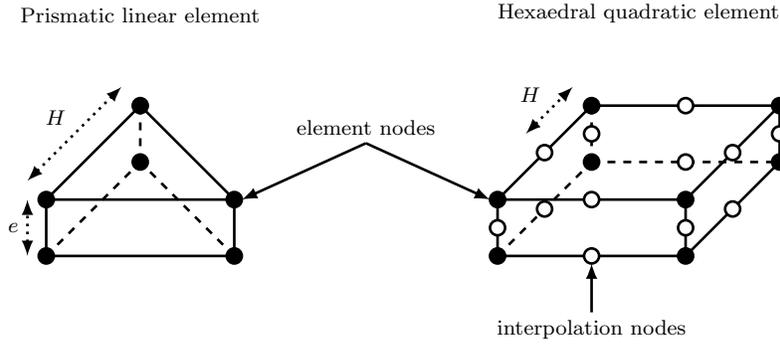
Figure 2: **Left:** Prismatic linear element where linear shape functions are defined between two element nodes. **Right:** Hexaedral quadratic element. Interpolation nodes are needed to define the quadratic shape functions.
