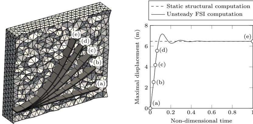
Figure 6: **Left:** Visualisation of the plate deformation within the fluid box. **Right:** Evolution of the maximal displacement of the plate extremity. The FSI computation is compared with the structural computation.
