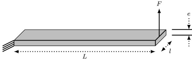
Figure 4: Geometrical parameters of the plate. The force  $F$  is applied over all the surface of the plate extremity.
