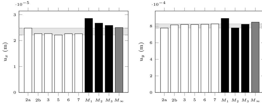
Figure 17:  $u_x$  and  $u_y$  components of the displacement of the beam extremity. The results obtained with the methods reported in [59] (displayed in white, and described in Tab. 6) can be compared with the present results, obtained for 3 different mesh resolutions (displayed in black). The extrapolated results are also provided (displayed in gray).
