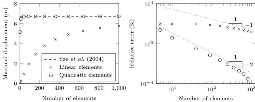
Figure 5: **Left:** Evolution of the maximal displacement as a function of the number of elements. Results obtained with both linear and quadratic hexaedral finite elements are compared with the result of Sze *et al.* (2004) [55]. **Right:** Error relative to most refined computation.
