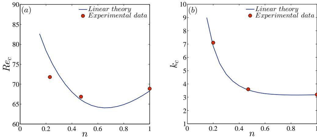
FIGURE 2: Comparison of theoretical (continuous line) and experimental (filled circle) variations of (a) the critical Reynolds number  $Re_c$  and (b) the axial wave number  $k_c$  as function of the shear-thinning effects  $n$ .
