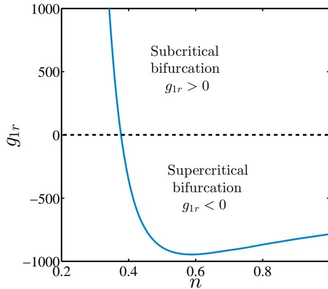
FIGURE 3: Evaluation of the real part of the Landau constant  $g_{1r}$  with a shear-thinning effects  $n$
