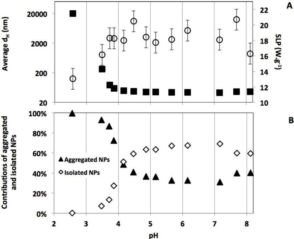
Figure 6: A: SLP (open circles – right scale) and hydrodynamic diameter,  $d_H$ , (filled squares-left scale) versus pH for PAA coated nanoparticles (maghemite mass fraction: 0.45 to 0.30 wt. %) – B: Relative contributions of isolated NPs ( $\%_{\text{isolated}}$ , open diamonds) and aggregates ( $\%_{\text{aggregated}}$ , triangles) versus pH
