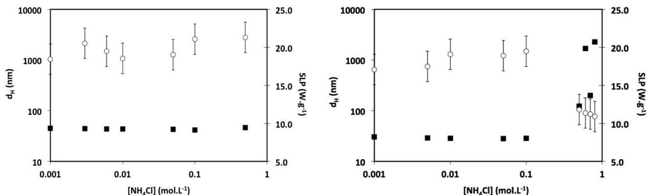
Figure 3: SLP (open circles – right scale) and hydrodynamic diameter,  $d_H$ , (filled squares – left scale) versus  $NH_4Cl$  concentration. Left: PAA coated NPs, right: PAAMA coated NPs, (maghemite mass fraction: 0.5 to 0.3 wt. %).
