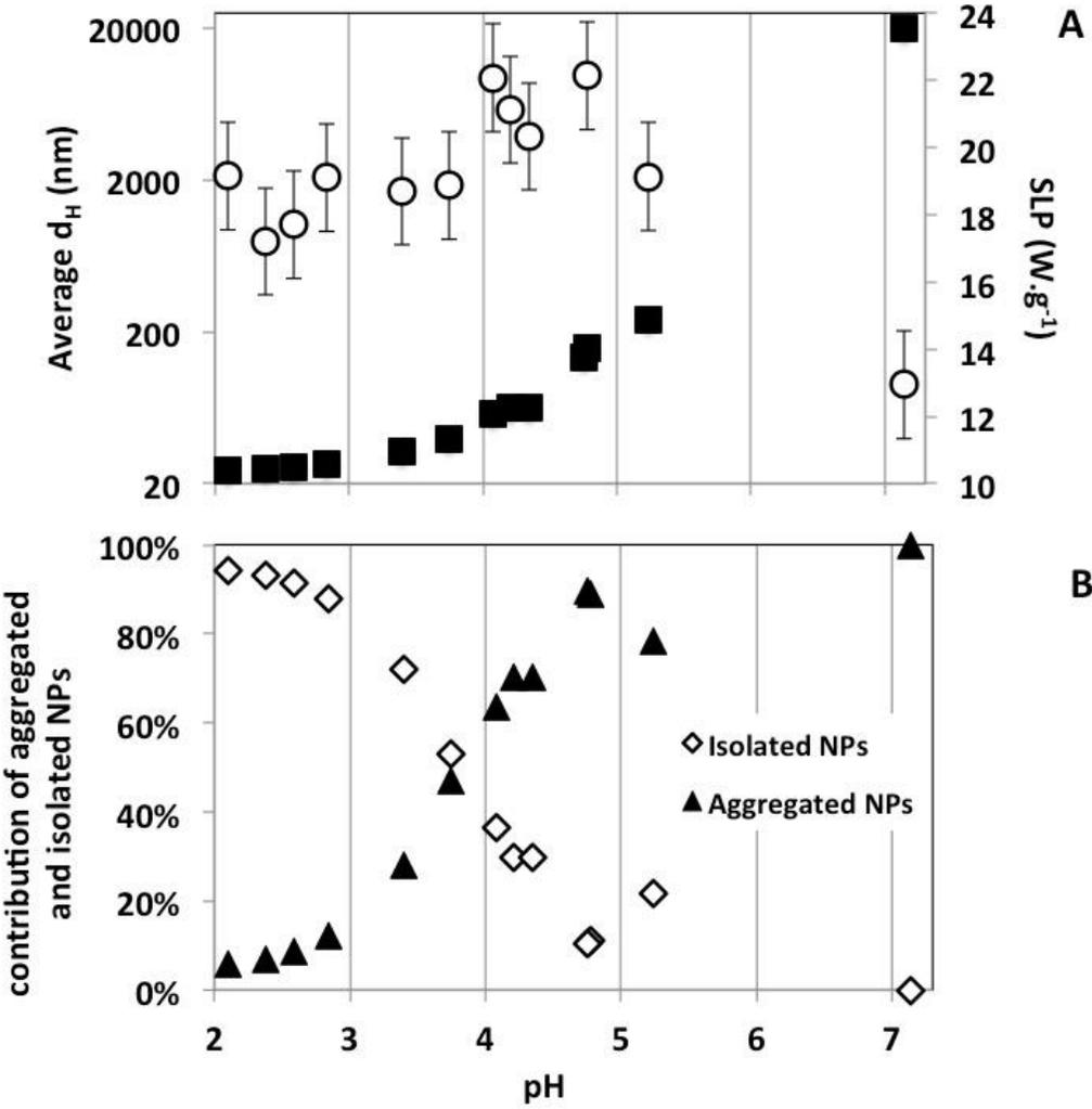
Figure 4: A: SLP (open circles-right scale) and average hydrodynamic diameter,  $d_H$ , (filled squares- left scale) versus pH for bare nanoparticles (maghemite mass fraction: 0.40 to 0.37 wt. %) – B: Relative contributions of isolated NPs (%<sub>isolated</sub>, open diamonds) and aggregates (%<sub>aggregated</sub>, triangles) versus pH
