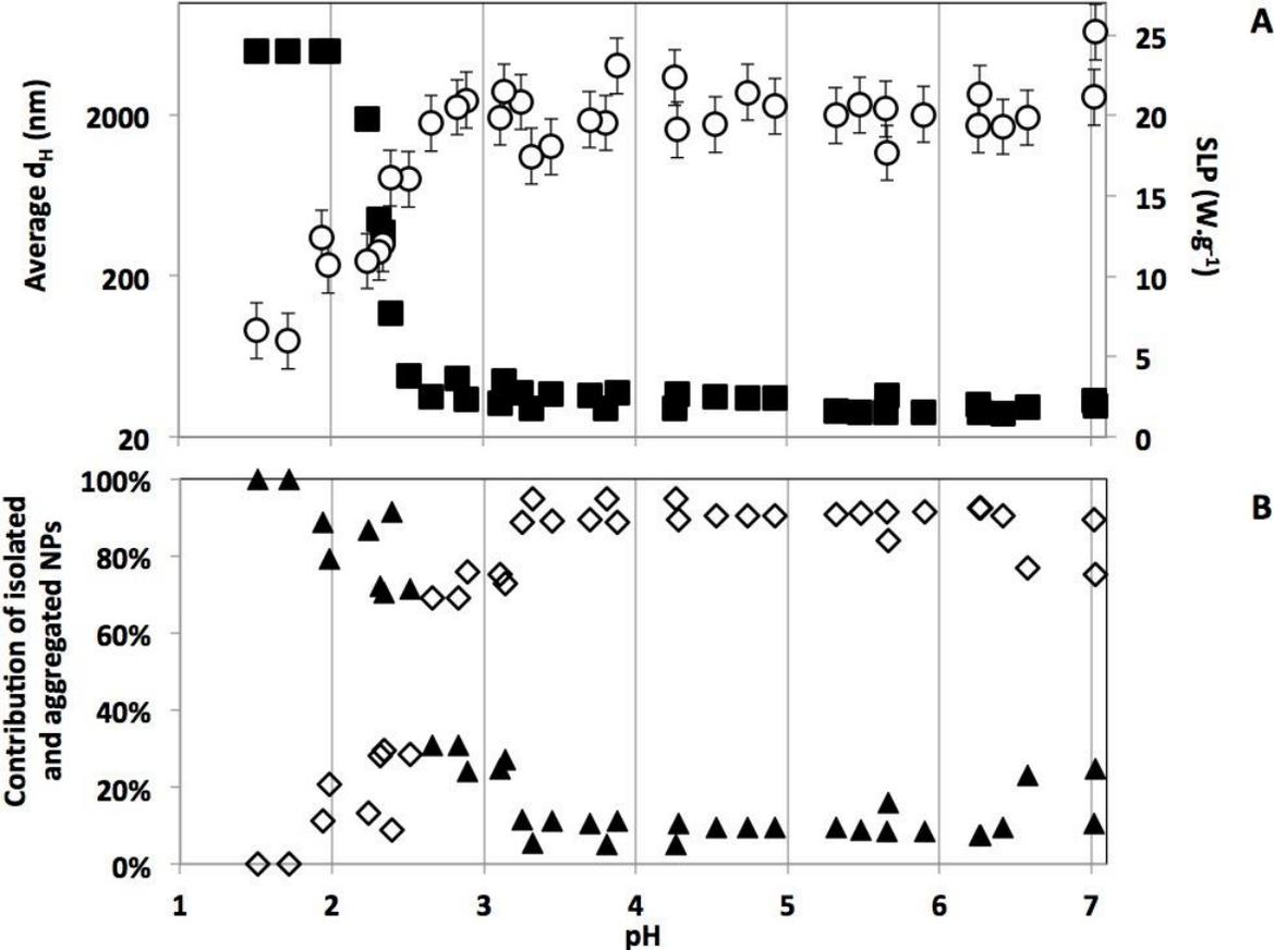
Figure 5 A: SLP (open circles – right scale) and averaged hydrodynamic diameter,  $d_H$ , (filled squares – left scale) versus pH for PAAMA coated nanoparticles (maghemite mass fraction: 0.45 to 0.30 wt%) – B: Relative contributions of isolated NPs ( $\%_{\text{isolated}}$ , open diamonds) and aggregates ( $\%_{\text{aggregated}}$ , triangles) versus pH
