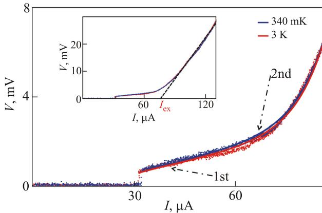
Fig. 2.  $I$ - $V$  characteristics measured on high- $J_c$  GB JJ (blue and red points refer to measurements at 340 mK and 3 K, respectively) are fitted according to Eqs. (6) and (7), which take into account both the RSJ model and vortex dynamics (blue and red line at 340 mK and 3 K, respectively). The inset shows the same  $I$ - $V$  curves in a wider range of current and voltage.
