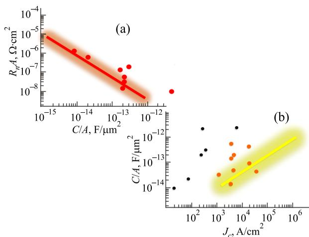
Fig. 4. (a) The orange curve gives the qualitative dependence of  $R_n A$  on  $C/A$ <sup>23,60,61</sup> for different types of HTS JJs. The red points come from SCD measurements on biepitaxial JJs,<sup>25,46,51</sup> (b)  $C/A$  vs  $J_c$ , the yellow curve represents data collected from literature.<sup>23,58-60</sup> Orange dots come from Refs. 26 and 27, while  $C/A$  values indicated by black dots are obtained through SCD measurements from Refs. 25, 46, and 51.
