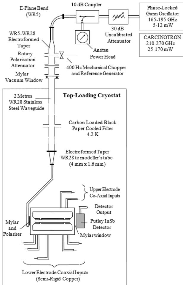
FIG. 8. Schematic diagram of the microwave system used.
