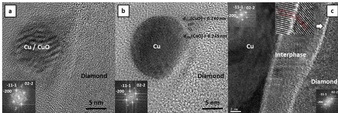
*Figure 5: High-resolution TEM micrographs of Cu particles deposited on diamond after nucleation and growth. (a) At the early stage of the exposure to the electron beam; (b) After having been exposed to the electron beam for several minutes; (c) Interface between the diamond surface and a deposited Cu particle.*
