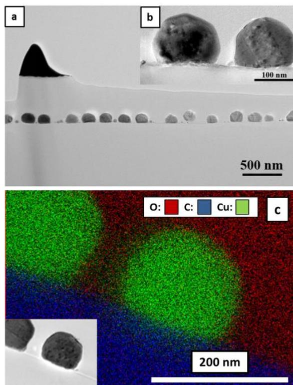
*Figure 4: (a) (b) TEM micrographs of a Cu-coated diamond surface; (c) EDS image of the Cu particles deposited on a diamond surface.*
