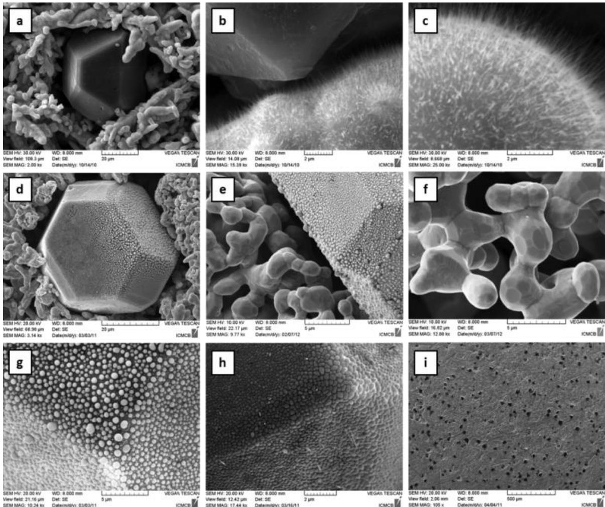
*Figure 2: SEM micrographs of a Cu/D(Cu) composite powder mixture. a) b) c) After debinding in air at 400°C and oxidation of copper; d) e) f) After reduction under Ar/H<sub>2</sub> at 400°C.*
