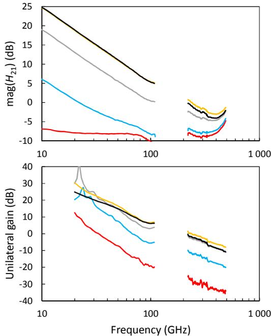
Fig. 6: Unilateral gain and Current gain H21 of a 2\*CBEB SiGe HBT of ( $0.22 \times 1 \mu\text{m}^2$ ) drawn emitter window size from Infineon for different  $V_{BE}$  ranging from 0.7-0.94 V with 60 mV step and  $V_{CB}=0$  V, using an on-wafer TRL calibration with impedance correction, plus move of the reference plane above vias at M6 (see Fig. 2).
