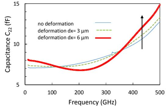
Fig. 15: Capacitance “C22” versus frequency of the transistor-open obtained from EM simulation including a TRL calibration with an ideal probe and with defaults ( $dx=3\mu\text{m}$ ,  $sx=6\mu\text{m}$ ) when simulating the transistor open.
