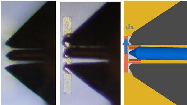
Fig. 14. Image of a 50  $\mu\text{m}$  pitch CPW probe a) before contact and b) after contact on a used ISS short standard. The probe flexibility in combination with a deteriorated ISS standard causes a deformation of the probe eventually modifying its characteristic impedance; c) Geometrical Model for EM simulation showing a default on CPW probe ( $dx=6\mu\text{m}$  movement at port 2).
