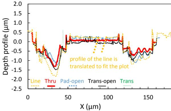
Fig. 11: Depth profile of the test structures (from Port 1 signal to Port 2 signal pads) after probing, highlighting probe positioning – measurement performed with an optical interferometer. Note that the profile of the line has been cut and has been translated to over-impose the profile at the pad position
