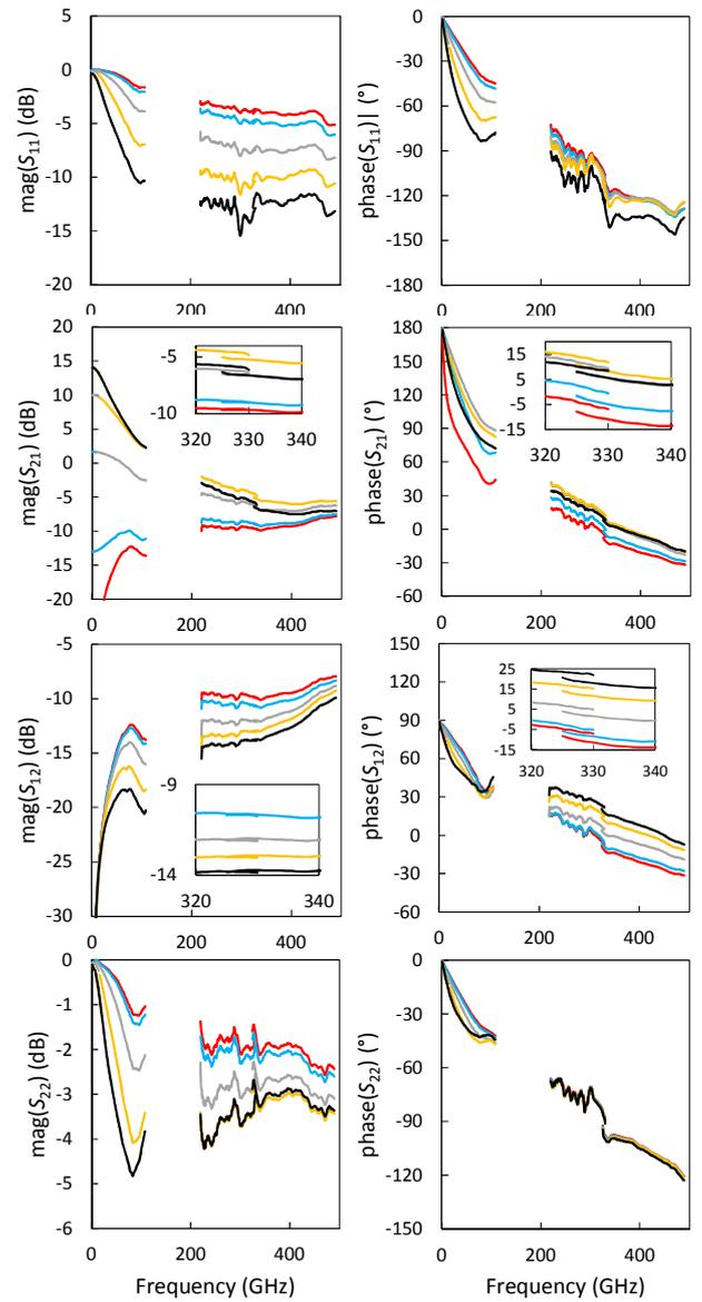
Fig. 7: S parameter measurements of a 2\*CBEB SiGe HBT of ( $0.22 \times 1 \mu\text{m}^2$ ) drawn emitter size from Infineon for different  $V_{BE}$  ranging from 0.7-0.94 V with 60 mV step and  $V_{CB}=0$  V, using an on-wafer TRL calibration with impedance correction and move of the reference plane above vias at M6 (see Fig. 2); magnitude and phase.
