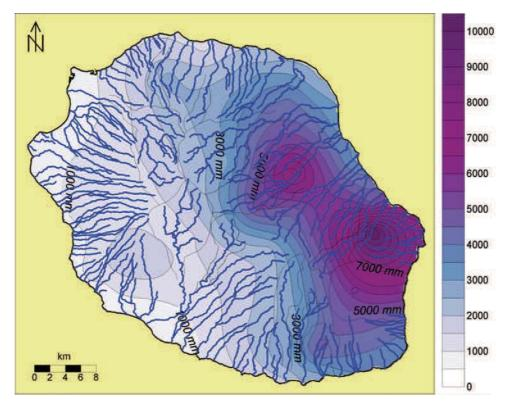
**Fig. 25.2** Mean annual precipitation (between 1971 and 2000) overlain by the hydrologic network for La Réunion. Isohyets have a contours spacing of 500 mm (Data from Meteo-France)
