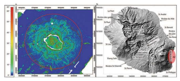
**Fig. 25.1** (a) Slope gradient computed from FOREVER and ERODER1 swath bathymetry and IGN DEM (1997) for the aerial part. *Brown lines* corresponded to -4,000, -3,000, -2,000 -1,000 and -500 m isobath. The *red circle* shows the approximate boundary between La Réunion and the abyssal plain. (b) Shaded relief map of Réunion Island showing
