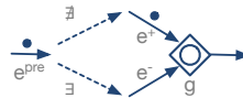
Fig. 3: Non activable inclusive gateway. It has to wait for the token on e^{pre} .
