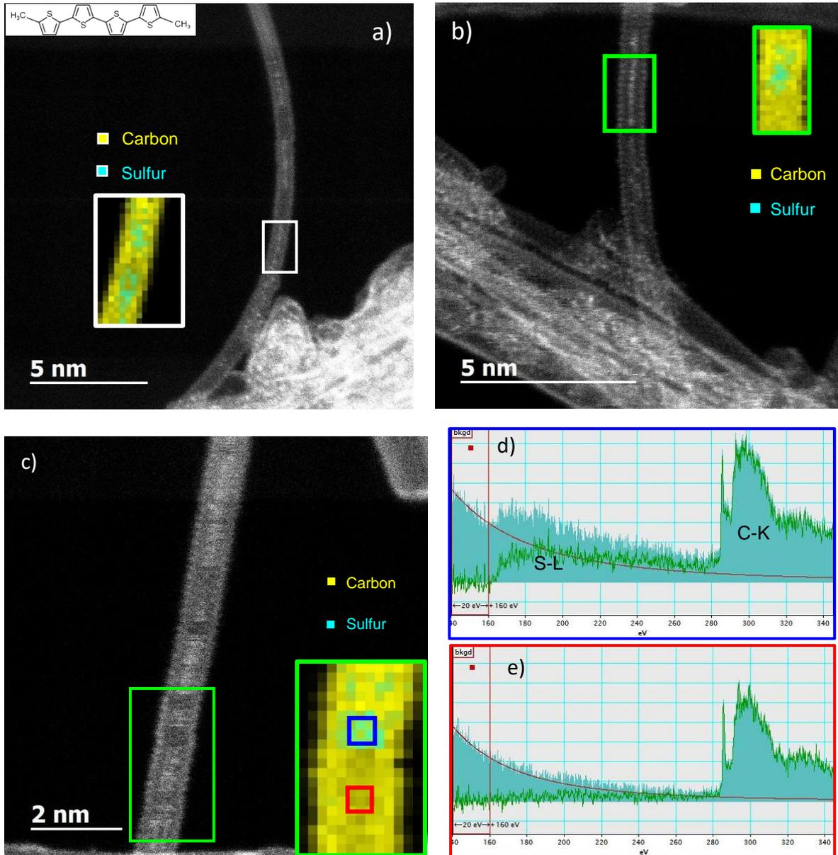
**Figure 1:** ADF-STEM images of a 4T@NT09 nanotubes and superimposed carbon (yellow) and sulfur (green) elemental maps. Two EEL spectra (d,e) extracted from the marked areas showing K edge of carbon ( $\sim 284$  eV) and  $L_{2,3}$  edge of sulfur ( $\sim 165$ – $220$  eV) only in (d). Inset in a) Structure of 4T.
