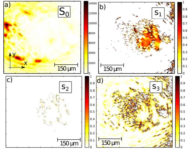
FIG. 3: Spatial mapping of the Stokes parameters of the reflected probe beam 1.5 ps after irradiation by the pump beam. a)  $S_0$  in color scale. b)  $s_1 = S_1/S_0$ . c)  $s_2 = S_2/S_0$ . d)  $s_3 = S_3/S_0$ .
