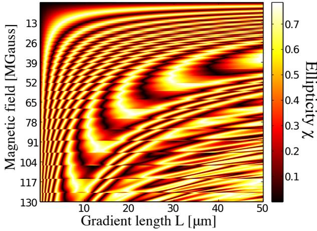
FIG. 6: Calculated change in polarization ellipticity after the back and forth path in a non-uniform plasma with an exponential density profile of gradient length  $L$  and a constant magnetic field. Results are obtained by solving the equations for the propagation of an electromagnetic wave inside of a magnetized plasma<sup>17</sup>.
