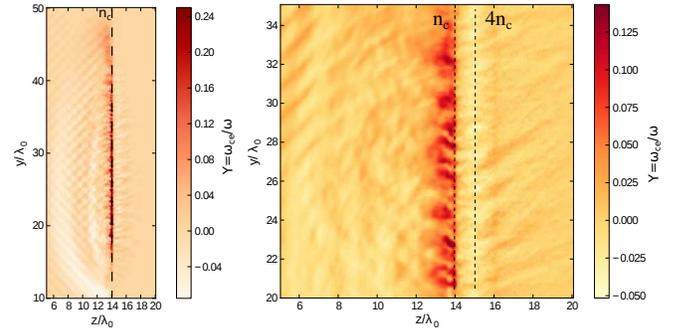
FIG. 8: a) PIC magnetic field map for the interaction of a  $4 \times 10^{17}$  W/cm<sup>2</sup> laser with a 1  $\mu$ m Al coating on a CH target, after 140 fs. b) Zoom of the interaction region.
