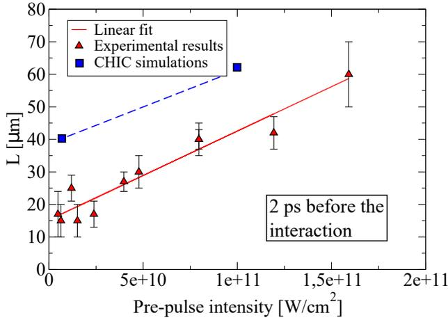
FIG. 2: Plasma density scale-length  $L$  at  $t = 2$  ps before the interaction of the main laser pulse, as a function of pedestal intensity. Triangles: experimental results from interferometry; continuous red line: linear fit of experimental results  $L = (2.7 \pm 0.2) \times 10^{-10} I_{\text{pre-pulse}} [\text{W}/\text{cm}^2] + (15 \pm 2) [\mu\text{m}]$ .
