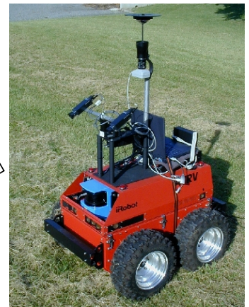
Fig. 8. Mobile robot ATRV Dala as a car-like robot: a nonholonomic system of dimension 4 with 2 nonholonomic constraints.
