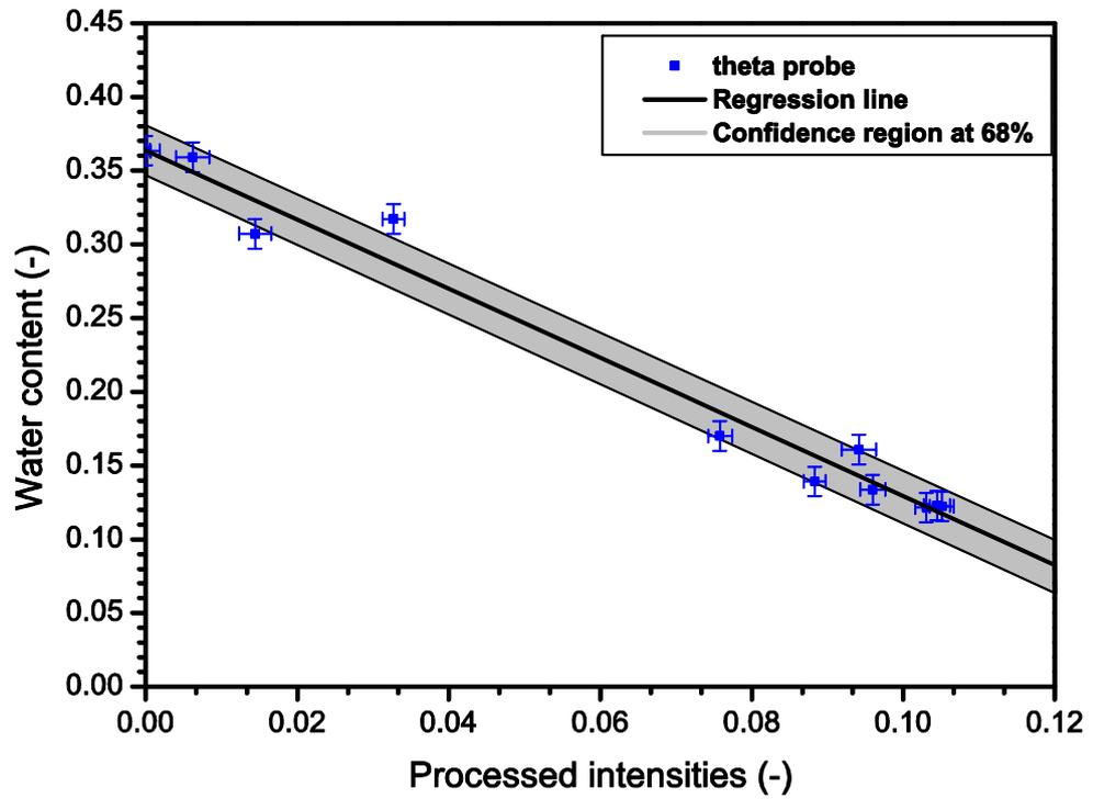
**Figure 3** Intensity vs. water content calibration plot of the theta probe installed in the validation flow tank; regression line and confidence intervals at 68 %. The horizontal and vertical bars correspond to the maximal measurement error on estimated to one standard deviation.
