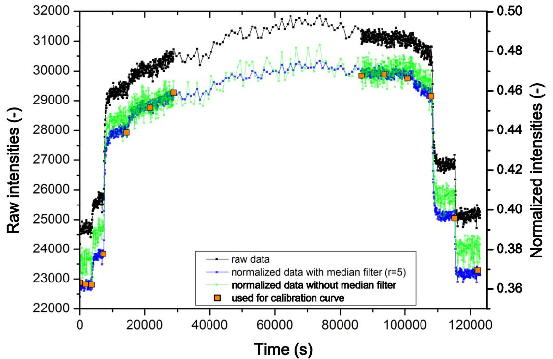
**Figure 2** Evolution of the mean intensity corresponding to the water content zone of measurement; black curve and symbols depict raw data, blue (green respectively) curve and symbols represent the normalized data after median filter (without median filter respectively). Orange squares correspond to the values used for the calibration curve construction.
