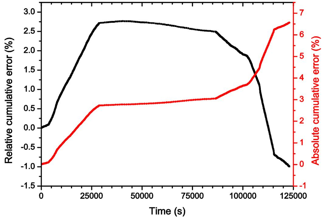
**Figure 4** Evolution of the error on water content in the flow tank: absolute cumulative error (red solid line, computed with Eq.[20]) and relative cumulative error (black solid line, computed with Eq.[21]) between measurements and computation.
