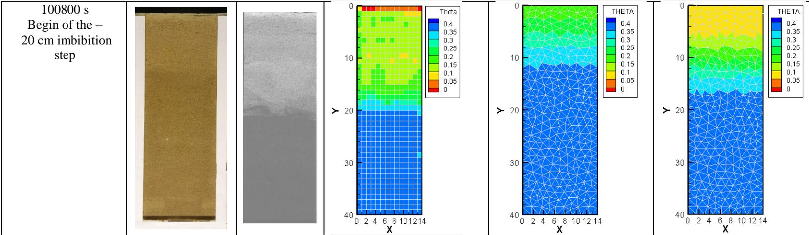
**Figure 7 Illustrations of the proposed photometric procedure. Images before and after treatment. Comparison of water content maps obtained through photometric procedure and numerical modelling (simulation 1 and 3).**
