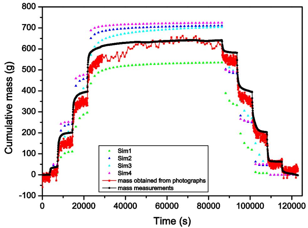
**Figure 6** Cumulative mass of water entering and leaving the validation flow tank during drainage / imbibition experiment: comparison of measured values (black symbols and line), values of photometric procedure (red symbols and line) and results of modelling (coloured triangles).
