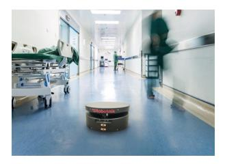
Fig. 1. The commercially available Robotnik RB1-base robot navigating in a healthcare environment
