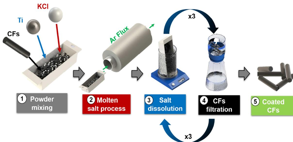
**Figure 2.** Schematic illustration of the molten-salt process for preparing TiC-based coatings on CFs.
