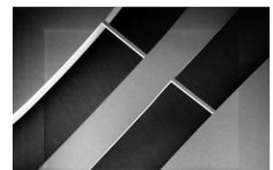
**Fig. 4** Microscopic image of the suspended waveguide
