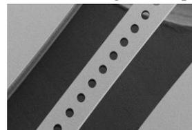
**Fig. 3** Microscopic image of the photonic crystal
