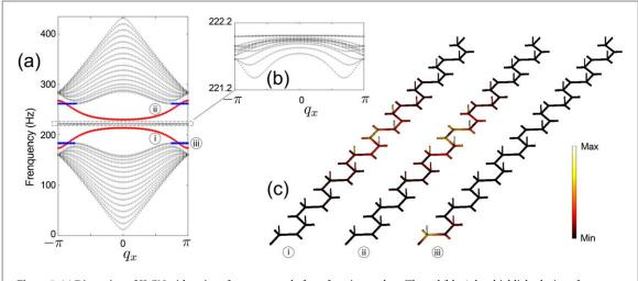
**Figure 5.** (a) Dispersion of SLGN with an interface composed of two free zigzag edges. The red (blue) dots highlight the interface (edge) mode branches. (b) Close view of the nearly flat region in (a). (c) Pressure field distributions of eigenmodes of the three bands in (a).
