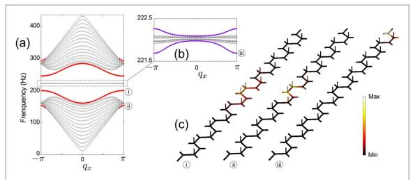
**Figure 4.** (a) Dispersion of SLGN with an interface composed of two resonant zigzag edges. The red dots highlight the interface mode branches. (b) Close view of the nearly flat region in (a). The edge wave branches are marked by magenta. (c) Pressure field distributions of eigenmodes corresponding to two red bands in (a) and a magenta band in (b).
