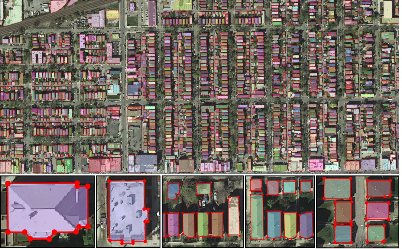
Figure 9. Extraction of buildings from satellite images with our algorithm: 1,178 buildings of a half square kilometer area of Chicago, USA, are extracted with low complexity polygons (8,683 vertices). While compact, the polygons capture some fine details (see closeups).
