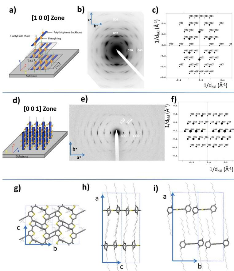
**Figure 5.** Comparison of the experimental and calculated ED pattern of highly oriented PDOPT thin films grown by epitaxy on naphthalene. a) - c) for the [100] zone (electron beam parallel to the octyl side chains) and d)-f) for the [001] zone (electron beam along the chain direction). a) and d) show schematic illustrations of the crystal orientations with respect to the electron beam (vertical). g)-i) are the typical projections of the refined structure of PDOPT
