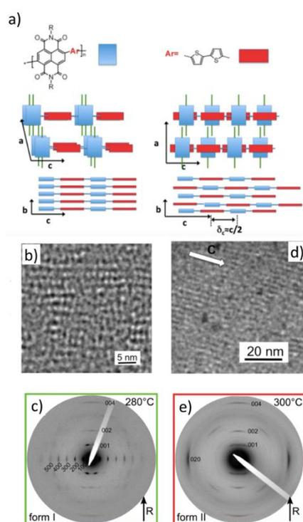
**Figure 6.** a) Schematic illustration of the stacking of NDI and T2 units for form I and II of P(NDI2OD-T2). b) HR-TEM of oriented thin films of P(NDI2OD-T2) obtained by directional epitaxial crystallization on TCB. c) Electron diffraction patterns of P(NDI2OD-T2) in form I
