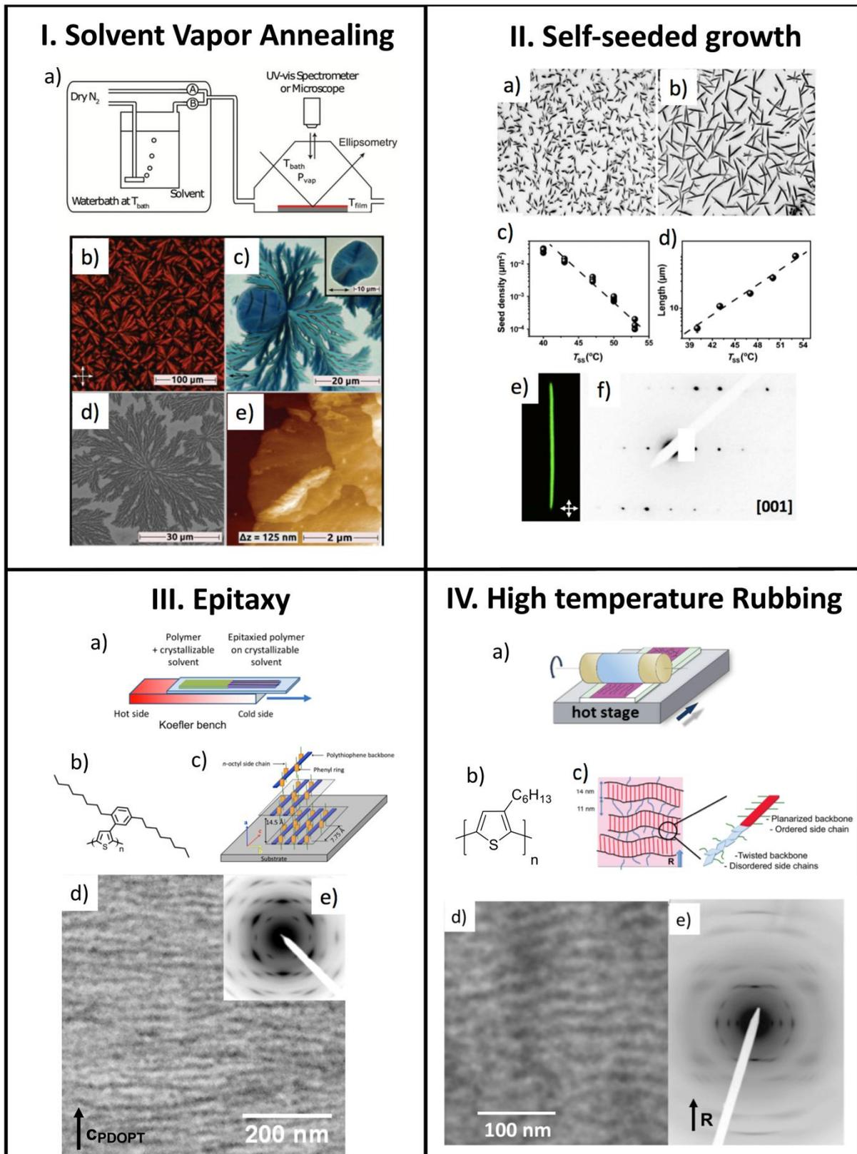
**Figure 2.** Comparison of four growth methods for polymer semiconductors: I) solvent vapor annealing. a) Schematic illustration of the experimental setup; b)–e) PCPDTBT films after CB-
