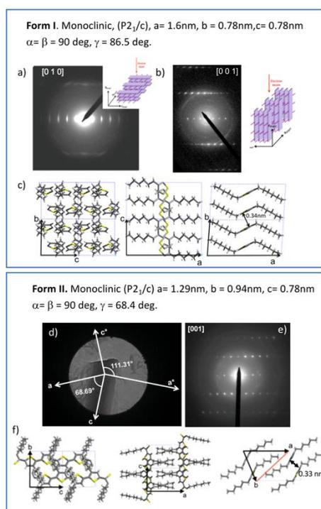
**Figure 4.** Comparison of the electron diffraction patterns of P3HT in oriented thin films of form I grown by epitaxy on TCB (a and b) and for a single crystal grown by self-seeding (e). In a) and b), the orientation of the electron beam with respect to the crystal is highlighted in the
