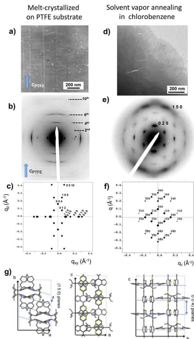
**Figure 8.** Bright field images (a, d), experimental ED patterns (b, e) and calculated ED patterns (c and f) using the refined structure shown in g) for PCPDTBT prepared by epitaxy on PTFE and solvent vapor annealing. g) Projections of the refined structure of PCPDTBT. Reproduced with permission from reference 64.
