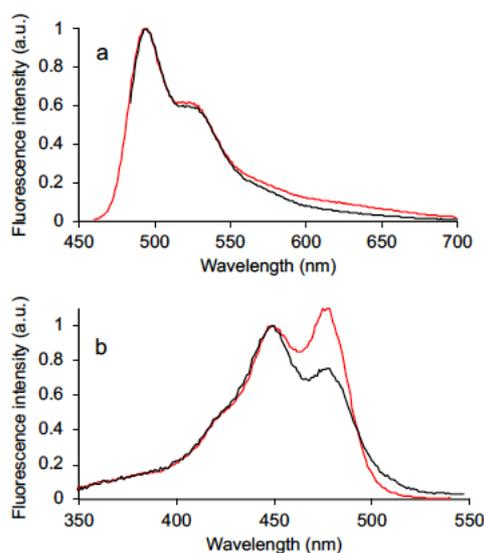
**Figure 5.** Steady-state fluorescence of **C8-Me**: a) fluorescence emission spectra obtained at  $\lambda_{\text{exc}} = 450$  nm (red line) and 475 nm (black line) and normalized to unity at the emission maximum; b) excitation spectra obtained at  $\lambda_{\text{obs}} = 550$  nm (red line) and 600 nm (black line) and normalized to unity at 449 nm. Concentration  $< 10^{-6}$  M in BE.
