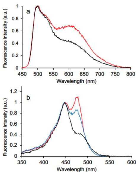
**Figure 4.** Steady-state fluorescence of **C6O2-Me**: a) fluorescence emission spectra recorded at  $\lambda_{\text{exc}} = 440$  nm (red line) and 465 nm (black line) and normalized to unity at the emission maximum; b) excitation spectra recorded at  $\lambda_{\text{obs}} = 650$  nm (black line), 550 nm (blue line) and 498 nm (red line) and normalized to unity at 449 nm. Concentration  $< 10^{-6}$  M in BE.
