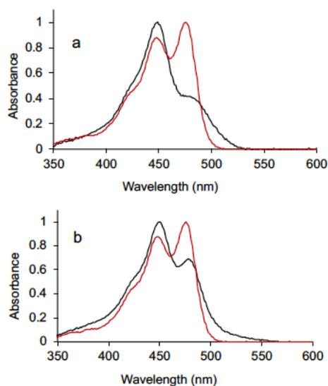
**Figure 3.** UV-Vis spectra of **R-Me** (red line) and of the bichromophoric compounds: a) **C6O2-Me** (black line) and b) **C8-Me** (black line). Concentration  $5 \times 10^{-7} - 10^{-6}$  M in BE. Spectra are normalized to unity at the absorption maximum.
