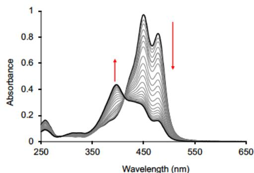
**Figure 7.** Changes in the UV-Vis spectrum of the EE solution of **C8-Me** upon irradiation with a continuous wave white light for different times. The final spectrum was obtained for an irradiation time of 1 hour. Concentration  $5 \times 10^{-6}$  M. The initial spectrum is normalized to unity at the absorption maximum.
