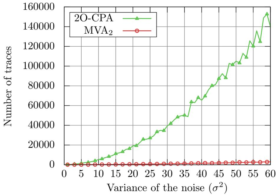
Fig. 3: Comparison between the number of traces to recover the key (with success probability of 80%) between the classical bi-variate attack and our multivariate attack (MVA<sub>2</sub>, meaning that it is rounded at degree 2)
