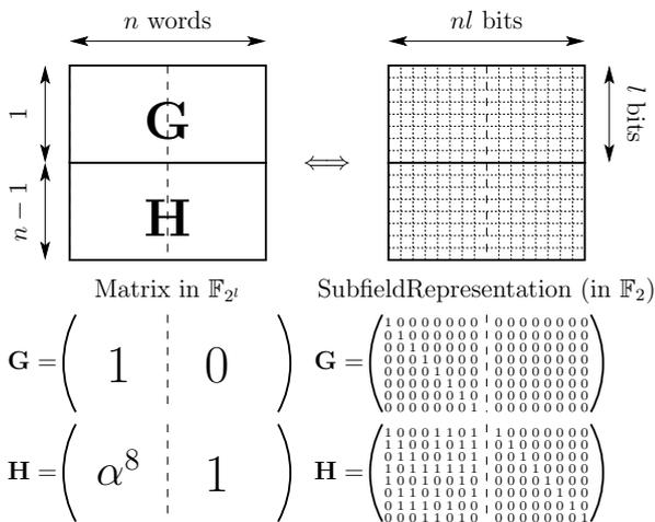
**Fig. 1** Dimensions of (typical) IPM encodings, for  $n = 2$ , on  $l = 8$  bits at byte-level. (Matrices  $\mathbf{G}$  and  $\mathbf{H}$  are examples.)
