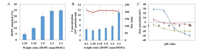
**Figure 3. Characterization of lipid-coated nanoMOFs.** (A) Quantification of the amount of DOPC in the nanoMOFs; (B) Mean hydrodynamic diameter (red) and concentration (blue) of DOPC-coated nanoMOFs determined by NTA. (C) Zeta potential of nanoMOFs as a function of pH before (blue) and after lipid coating with (red) or without (green) the addition of DSPE-PEG 2000.
