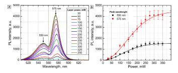
Fig. 3. Two-photon-excited photoluminescence (PL) spectra of the CdSe(core)/ZnS/CdS/ZnS(multishell) quantum dots (QDs) inside the porous silicon microcavity. (a) PL spectra of the QDs inside the microcavity under two-photon excitation at various laser pump powers. (b) The corresponding PL intensity dependences on the pump power at 575 nm (red) and 550 nm (black).
