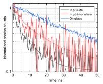
Fig. 4. The experimental (solid lines) and fitted (dashed lines) twophoton-excited PL decay of the QDs embedded in the porous silicon microcavity (black), embedded in the monolayer (red), and deposited onto a glass substrate (blue).
