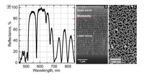
Fig. 1. The reflectance spectrum of the porous silicon microcavity (a) and scanning electron microscopy images of the cross-section (b) and the surface (c) of the fabricated porous silicon microcavity.
