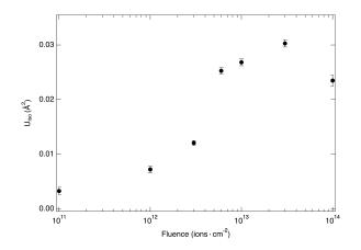
FIG. 6. Thermal displacement parameters (Uiso) as a function of fluence for pristine and 92 MeV Xe irradiated  $Sc_4Hf_3O_{12}$ . Uiso parameters were obtained after Rietveld refinement and indicates an increase of disorder in the  $\delta$ -phase which gradually saturates when the structure is transformed to a defect fluorite phase.
