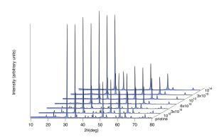
FIG. 4. x-ray diffraction patterns obtained from pristine and 92 MeV Xe irradiated  $Sc_4Hf_3O_{12}$  at fluences ranging from  $10^{12} - 10^{14}$  Xe/cm<sup>2</sup>. The vanishing of superlattice reflections characteristic of the trigonal  $\delta$ -phase occurs above  $6 \times 10^{12}$ Xe/cm<sup>2</sup>. Before that apparent long-range symmetry changes, the intensity of those superlattice reflections decreases continuously due to a progressive change in the crystal structure.
