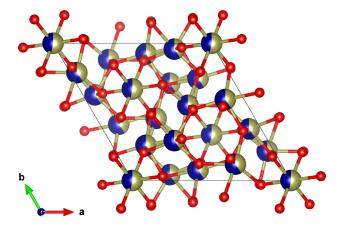
FIG. 3. 3D ball and stick structural model of  $Sc_4Hf_3O_{12}$  projected along the c-axis. The dual colored atoms display cations with a fractional occupancy of Sc (Blue) and Hf (Gold).
