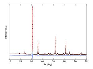
FIG. 2. Observed (black dots), calculated (red solid line) XRD pattern for pristine  $\delta$ -Sc<sub>4</sub>Hf<sub>3</sub>O<sub>12</sub> showing a good Rietveld refined fit with the structural model shown in table I. The blue solid line indicates the difference between the observed and calculated patterns.
