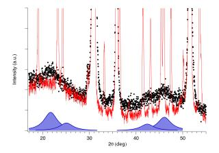
FIG. 7. XRD patterns obtained from  $Sc_4Hf_3O_{12}$ , pristine delta phase (solid red) and irradiated with  $10^{14}$  Xe/cm<sup>2</sup> (black dots) showing emergence of diffuse scattering (blue peaks) at the angular positions corresponding to (211), (220), (332), and (413) superlattice reflections of bixbyite-related structures (Ia3,  $a_B=2a_F$ )
