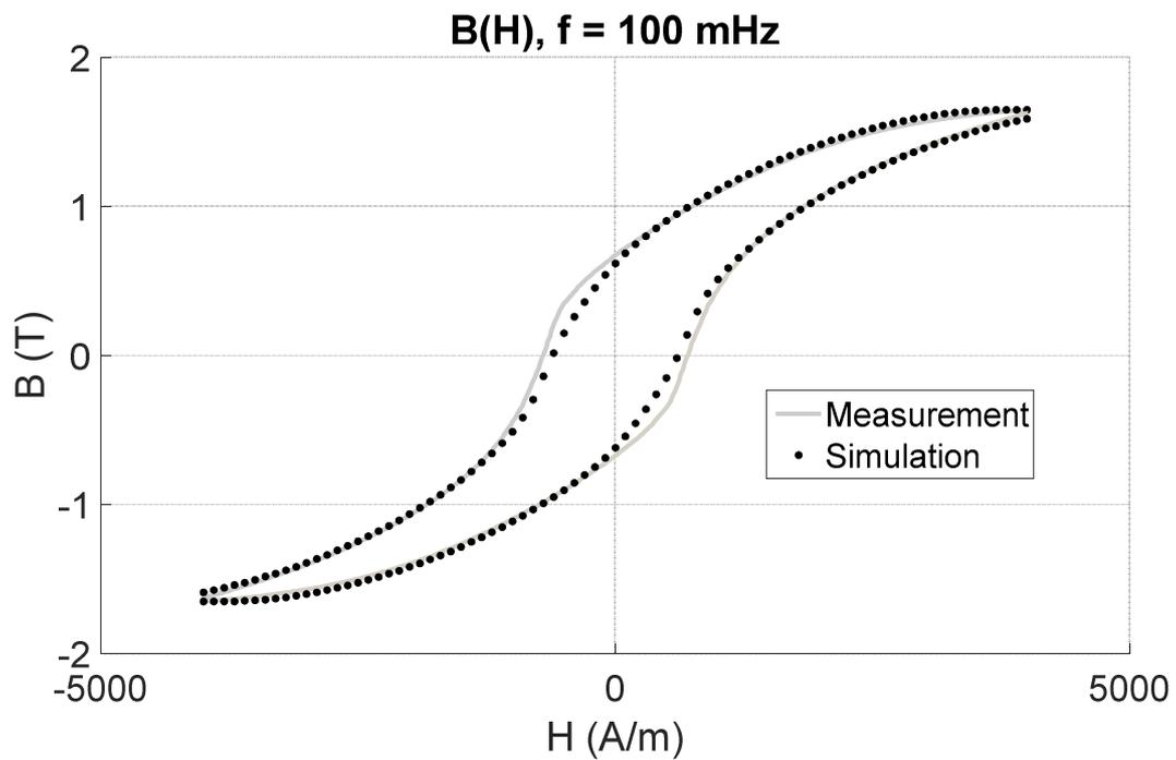
Fig. 8 – Comparison simulation/measure under quasi-static magnetic field excitation.
