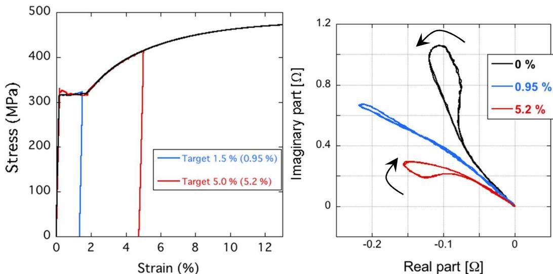
Fig. 1 – Experimental EC-MS signatures under different mechanical stress level [10].
