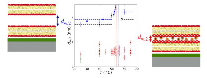
Figure 1: Schematics of the deposited double bilayer. For zwitterionic bilayers (left), charged bilayers (right). The water layer between bilayers is thinner for charged bilayers (center). (Figure courtesy of Mukhina et al.)
