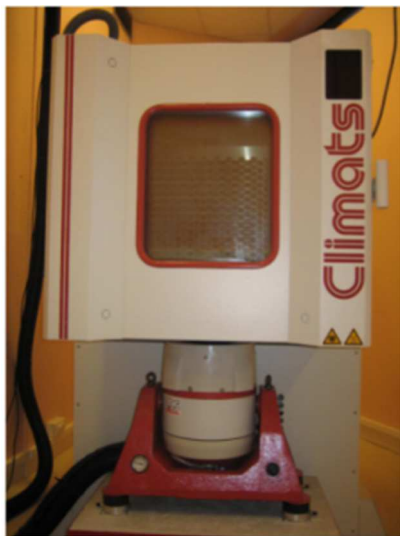
Fig. 1. Thermal chamber associated with a vertical vibration
