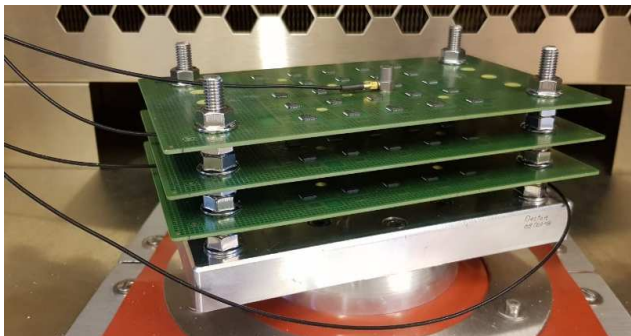
Fig. 5. Boards mounting and accelerometers fixing
