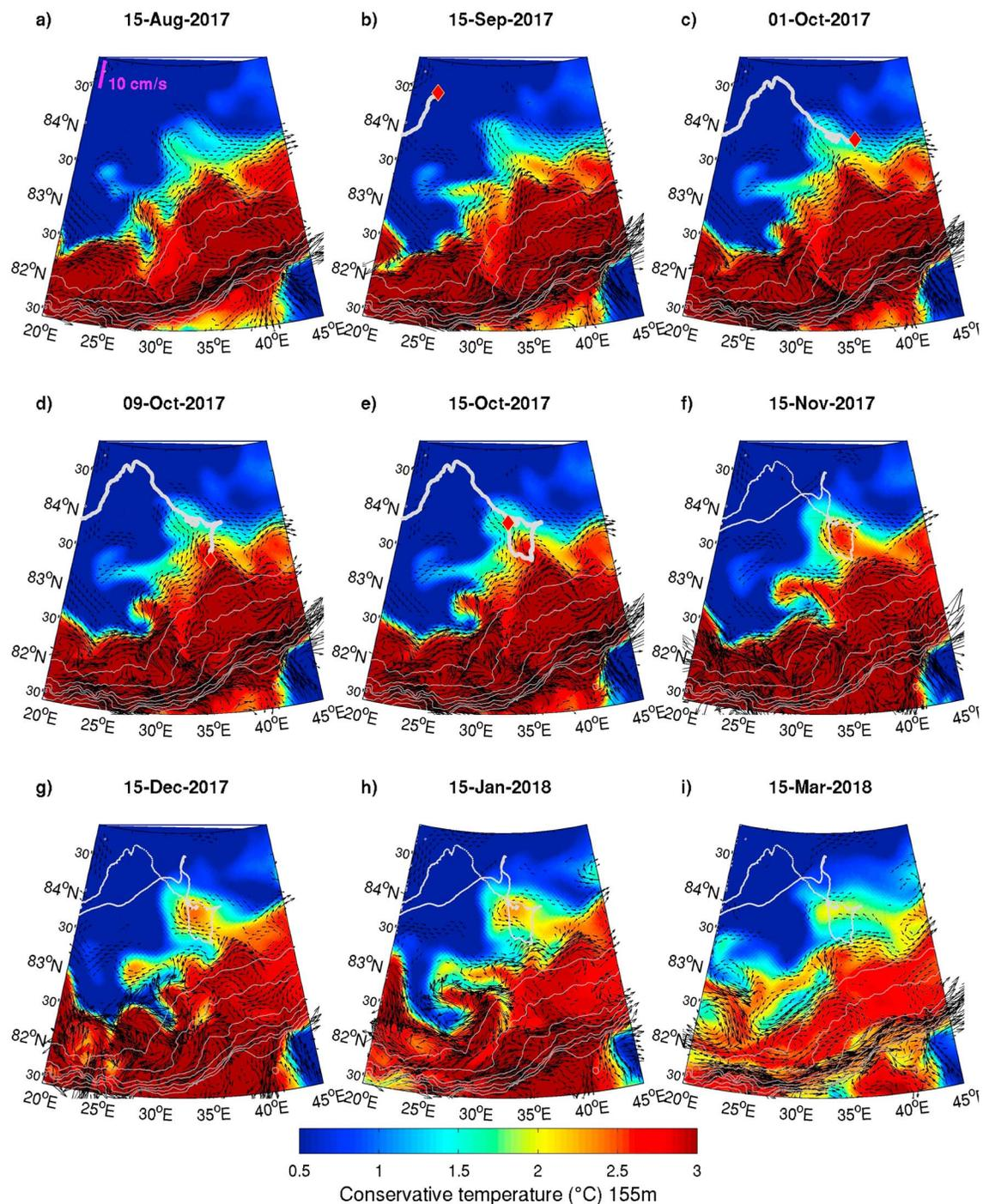
**Figure 12.** Selected snapshots of the Atlantic Water mesoscale structure in Mercator Ocean model outputs shown at 155 m. The white line corresponds to the Ice Atmosphere Ocean Observing System platforms trajectory. The red diamond marks the position of the platforms at each selected date. Gray isolines are bathymetry contours. Black arrows are the current at 155 m in the model; the scale is indicated in (a). Velocities lower than 1 cm/s are not shown.
