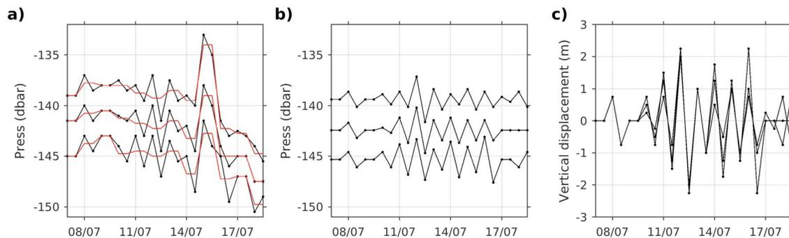
**Figure A1.** (a) Example of three sample isopycnals over a 12-day period (7 to 18 July 2017, over the Gakkel Ridge). The black lines show the depth of the isopycnals, and the red line shows the daily mean depth of the three isopycnals. (b) The same isopycnals with the mean removed, leaving only displacements near the inertial frequency. (c) Vertical displacements of the three isopycnals combined to maximize the number of points available.
