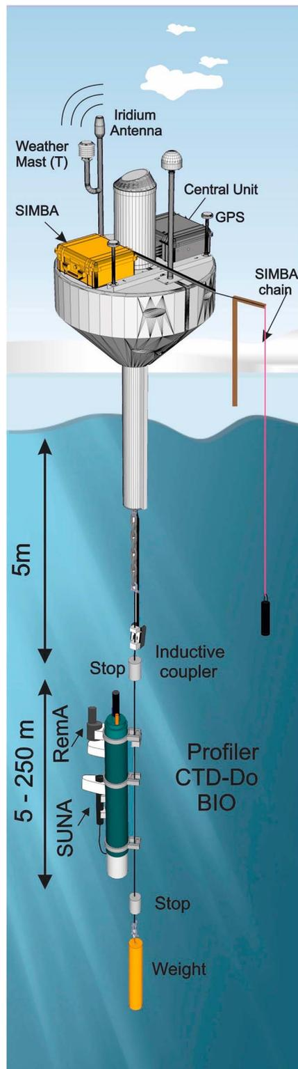
**Figure 1.** Schematic of IAOOS platform 24. The ocean profiler was equipped with bio-optics sensor suite (pack Rem-A) and a nitrate sensor (SUNA) in addition to the traditional CTD-DO sensors. SIMBA = Scottish Association for Marine Sciences ice mass balance for the Arctic; CTD = conductivity, temperature, and depth; SUNA = submersible ultra-violet nitrate analyzer.
