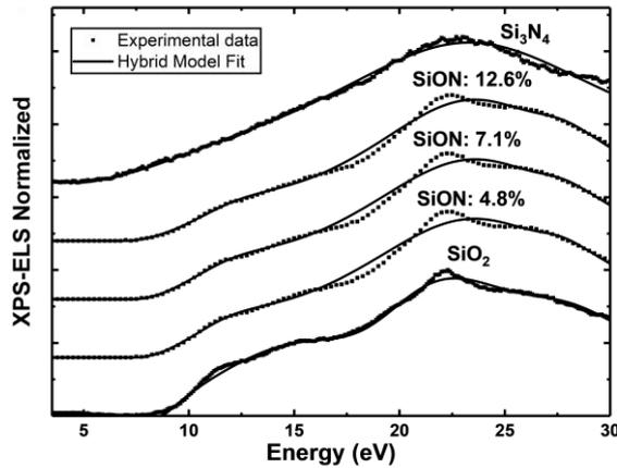
Figure 3 XPS-ELS experimental and simulated data after the main peak for the  $\text{SiO}_2$ - $\text{Si}_3\text{N}_4$  thin films. Scattered points denote the experimental data and the lines denote the triple oscillator Tauc-Lorentz model that couples ellipsometry measurements the XPS-ELS data. All spectra represent the ELS after the O1s main core peak, except the  $\text{Si}_3\text{N}_4$  where the N1s ELS is pictured.
