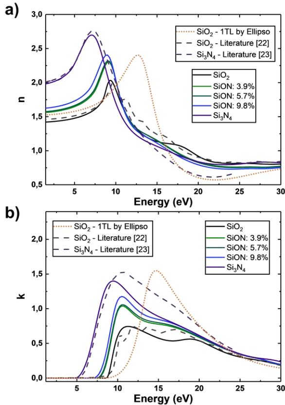
Figure 5 Modelled optical properties with the energy for the SiO<sub>2</sub>-Si<sub>3</sub>N<sub>4</sub> thin films between 1.5 and 30 eV. a) Refractive index,  $n$ , and b) coefficient of extension  $k$ . Literature curves of SiO<sub>2</sub> and Si<sub>3</sub>N<sub>4</sub> are represented with dashed lines. References: SiO<sub>2</sub>[27] and Si<sub>3</sub>N<sub>4</sub>[28]
