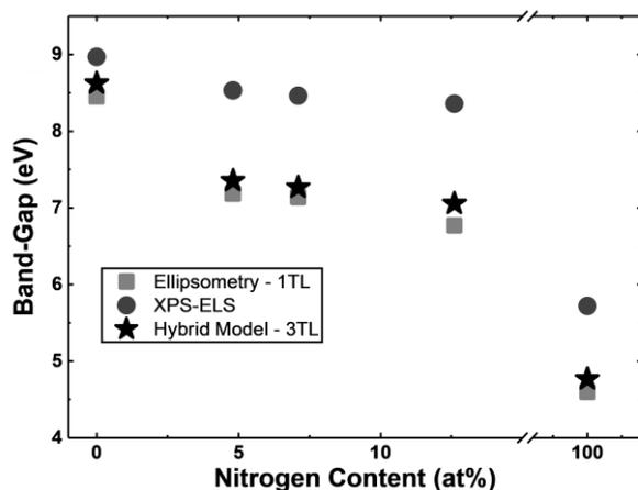
Figure 4 Bandgap energy dependency with the nitrogen content in  $\text{SiO}_2\text{-Si}_3\text{N}_4$  thin films. Comparison of each technique separately (Ellipsometry and XPS-ELS) and the hybrid method for a triple oscillator Tauc-Lorentz model
