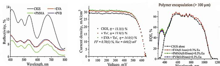
The reflectance spectra as well as V-I curves registered for the cells with LDS layer composed of Eu(III) luminescent complex with the highest QY. EQE plots for the CIGS without and with LDS layers encapsulated in different types of polymers.
