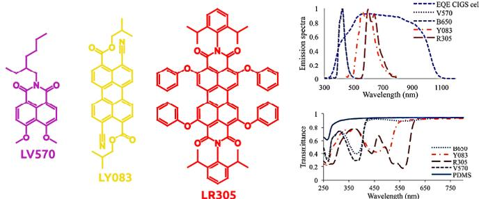
The chemical structures of lumogen family compounds incorporated into PMDS polymer matrix, together with emission and transmittance spectra of the LDS thin films at room temperature.
