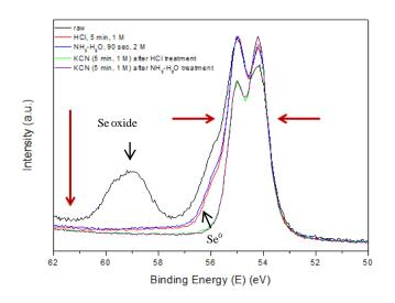
Fig. 2.  $Se_{3d}$  photopeaks acquired on CIGS surfaces of an aged as grown sample (black) and after different chemical treatments of this surface (HCl, NH<sub>3</sub>-H<sub>2</sub>O, HCl-KCN and NH<sub>3</sub>-H<sub>2</sub>O-KCN).
