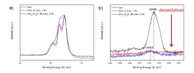
Fig. 1. a)  $Ga_{3d}$ -In<sub>4d</sub> and b)  $O_{1s}$  photopeaks acquired on CIGS surfaces (on soda-lime substrate) of an aged raw sample (black) and after treatment of this surface by a subsequent HCl dipping (red) or a  $NH_3$ - $H_2O$  (blue) dipping.
