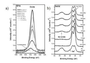
Fig. 3. Time evolution of CIGS deoxidized surfaces: a)  $O_{1s}$  and b)  $Se_{3d}$  (after HCl+KCN treatment) photopeaks acquired just after treatment until 4 months air ageing. The as-grown spectra are shown for comparison.
