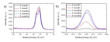
Fig. 4. a)  $Se_{3d}$  and b)  $Na_{1s}$  photopeaks evolution over air ageing for a rinsed CIGS sample deposited on flexible substrate with NaF post-deposition treatment.
