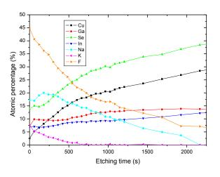
Fig. 5. XPS atomic percentage evolution over etching time for the different elements present in the CIGS sample.
