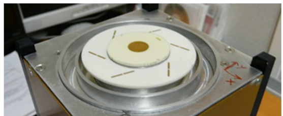
Fig. 8. The manufactured antenna is integrated on top of a 3U platform
