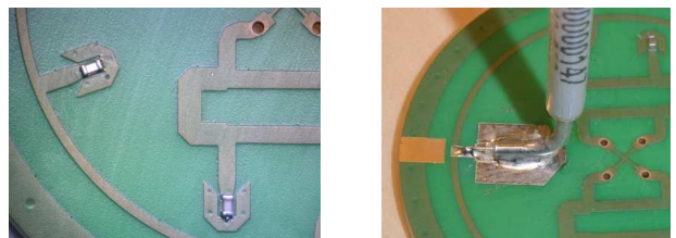
Fig. 7. SMD components and coaxial cable are soldered on the circuit.
