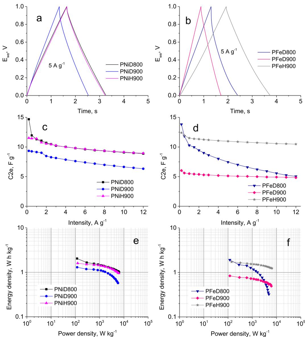
**Fig. 5.** Galvanostatic charge–discharge (GCD) results obtained with 2 mol L<sup>-1</sup> H<sub>2</sub>SO<sub>4</sub> electrolyte within the potential window 0–1 V: (a,b) GCD curves recorded at 5 A g<sup>-1</sup>; (c, d) Specific capacitance values from 0.2 to 12 A g<sup>-1</sup>; (e,f) Ragone plots.
