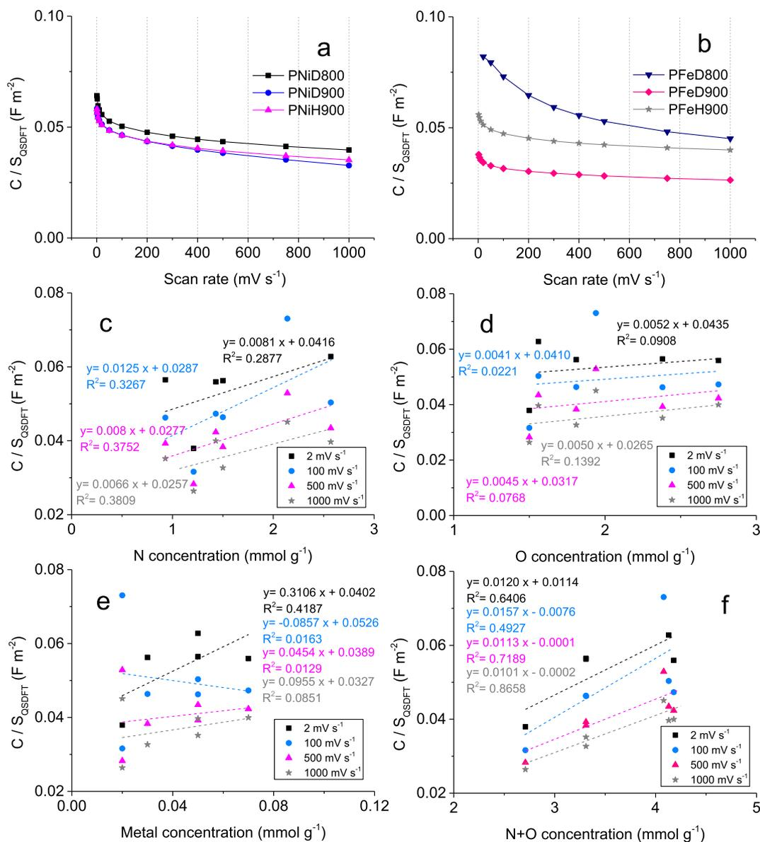
**Fig. 6.** (a,b) Interfacial capacitance,  $C/S_{QSDFT}$ , obtained from CV curves at scan rates between 1 and 1000 mV s<sup>-1</sup>; (c–f) Interfacial capacitance vs surface concentration of heteroatoms (N, O, metal, and N + O).
