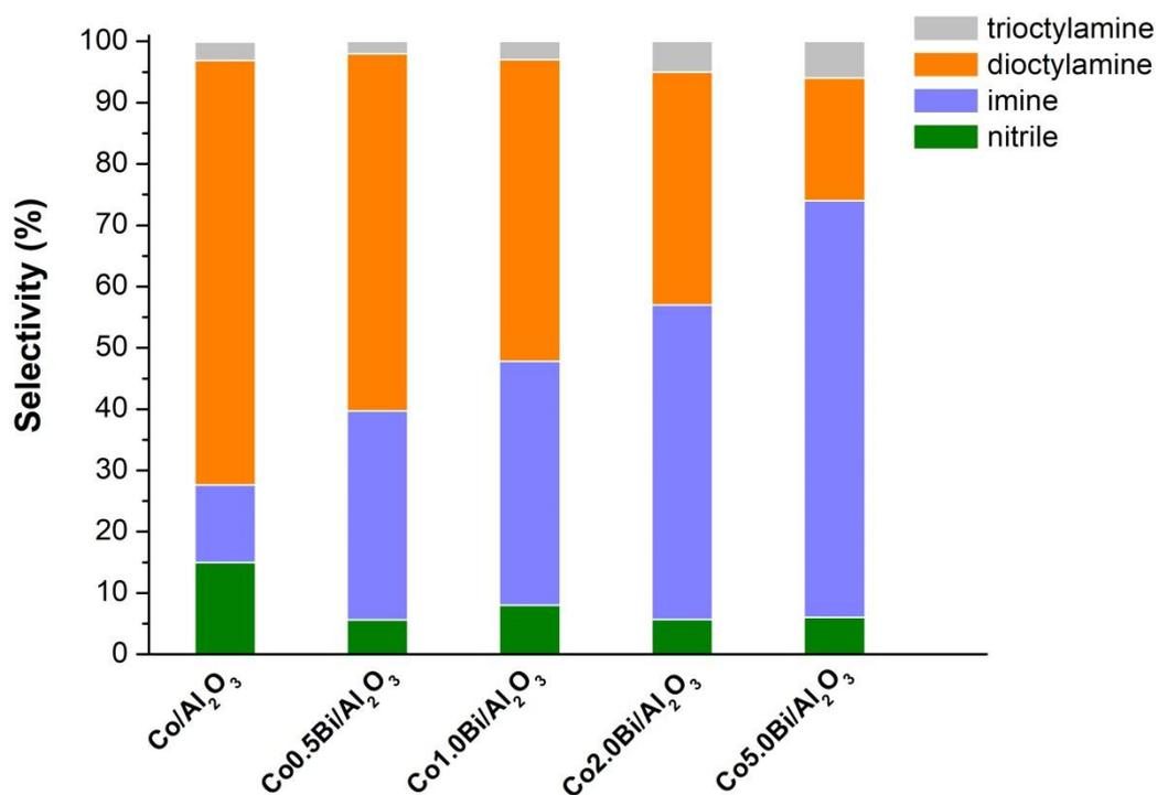
**Figure 8** Model reaction of 1-octylamine transformation over activated Co/Al<sub>2</sub>O<sub>3</sub> and bimetallic Co<sub>x</sub>Bi/Al<sub>2</sub>O<sub>3</sub> catalysts at a conversion of < 10% (1-octylamine, 1 mL; catalyst amount, 20 mg; molar ratio of 1-octanol/NH<sub>3</sub>/H<sub>2</sub> = 1/4.5/0.85; P<sub>H<sub>2</sub></sub> = 3 bar; reaction temperature, 180 °C; time, 0-4 h; no solvent used).
