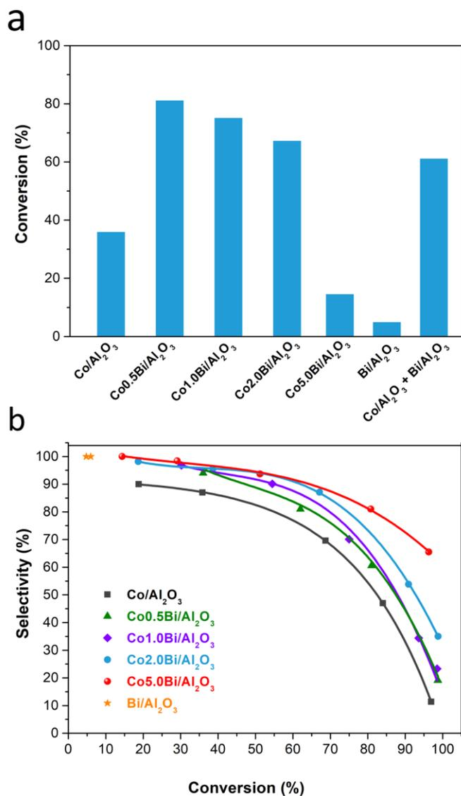
**Figure 3** Catalytic conversion modification by Bi promotion (a) and selectivity-conversion curves (b) for liquid phase amination of 1-octanol over activated Co/Al<sub>2</sub>O<sub>3</sub> and bimetallic Co<sub>x</sub>Bi/Al<sub>2</sub>O<sub>3</sub> catalysts (1-octanol, 0.84 g; molar ratio of 1-octanol/NH<sub>3</sub>/H<sub>2</sub> = 1/4.5/0.85; P<sub>H<sub>2</sub></sub> = 3 bar; catalyst amount, 100 mg; reaction temperature, 180 °C; time, 0-48 h; no solvent used).
