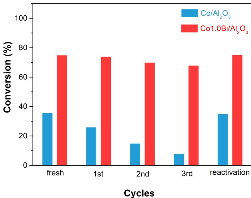
**Figure 4** Catalytic reusability and stability for liquid phase amination of 1-octanol over activated Co/Al<sub>2</sub>O<sub>3</sub> and Co1.0Bi/Al<sub>2</sub>O<sub>3</sub> catalysts (1-octanol, 0.84 g; molar ratio of 1-octanol/NH<sub>3</sub>/H<sub>2</sub> = 1/4.5/0.85; P<sub>H<sub>2</sub></sub> = 3 bar; catalyst amount, 100 mg; reaction temperature, 180 °C; time, 5 h; no solvent used; reactivation condition: 400 °C calcination under air followed by H<sub>2</sub> activation at 450 °C).
