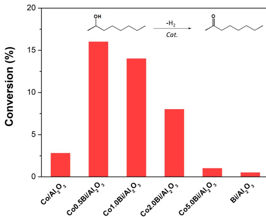
**Figure 7** Comparison of catalytic conversion for liquid phase dehydrogenation of 2-octanol over activated Co/Al<sub>2</sub>O<sub>3</sub>, Bi/Al<sub>2</sub>O<sub>3</sub> and bimetallic Co<sub>x</sub>Bi/Al<sub>2</sub>O<sub>3</sub> catalysts (2-octanol, 50 mg; toluene, 1 g; catalyst amount, 50 mg; reaction temperature, 140 °C; time, 15 h).
