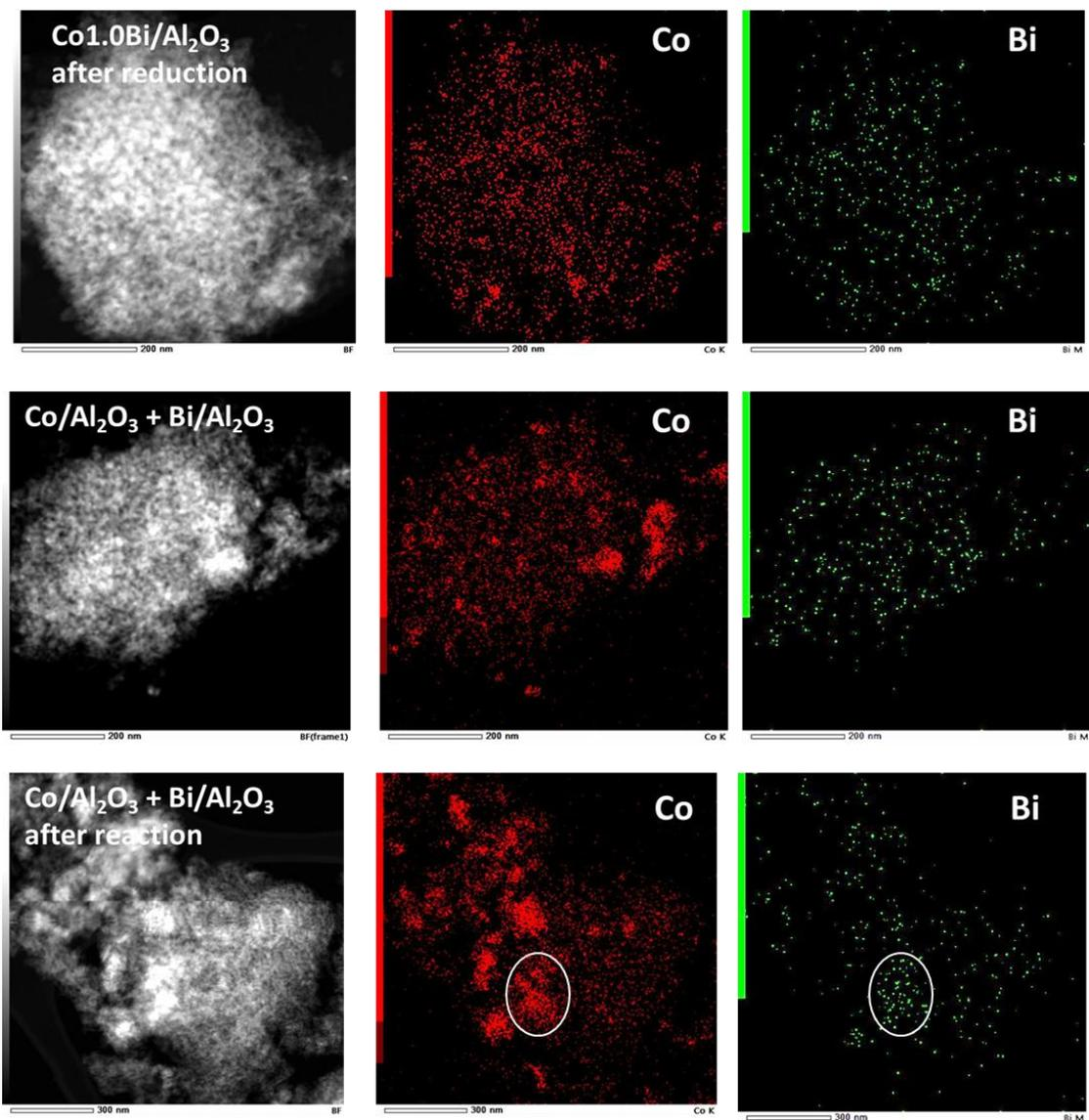
**Figure 6** HAADF-STEM images and EDX mapping of Co and Bi of reduced  $\text{Co}_{1.0}\text{Bi}/\text{Al}_2\text{O}_3$  catalyst and mechanical mixture  $\text{Co}/\text{Al}_2\text{O}_3 + \text{Bi}/\text{Al}_2\text{O}_3$  before and after reaction of amination
