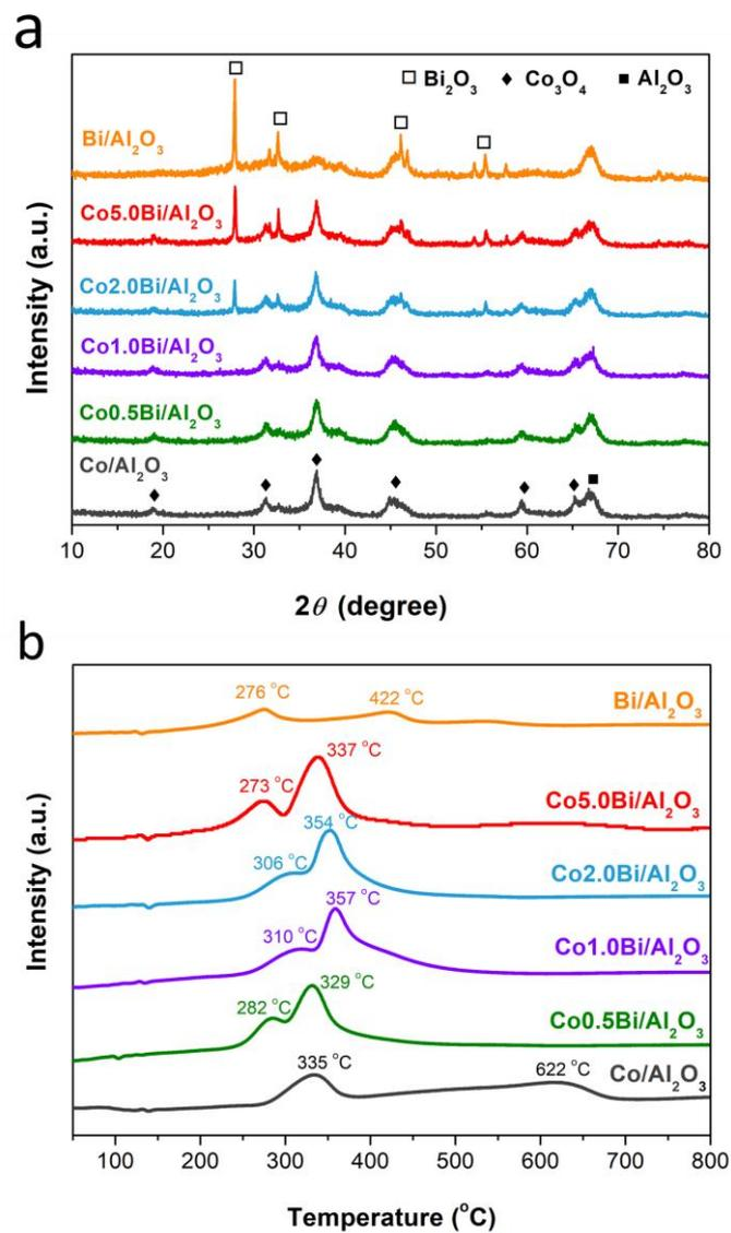
**Figure 5** XRD patterns (a) and H<sub>2</sub>-TPR profiles (b) of oxidized Co/Al<sub>2</sub>O<sub>3</sub>, Bi/Al<sub>2</sub>O<sub>3</sub> and bimetallic Co<sub>x</sub>Bi/Al<sub>2</sub>O<sub>3</sub> catalysts.
