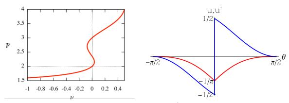
Fig. 7 Left:Value of the exponent p of a singularity of the type  $r^p u(\theta)$  for  $U^0$  at a corner of the plate in function of the Poisson ratio  $\nu$ . When p < 2, then  $U^0$  is not regular enough in order that  $U^1$  be in  $H^2(\Omega_0)$ . It is the case when  $-1 < \nu < 0$ . Right: angular function u (red) and its derivative u' (blue) entering in the singular part of  $U^1$  at the end points  $\mathbf{D} \pm$  of the line of defect.
