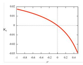
Fig. 2 Graphs of the two coefficients  $C_c$  and  $K_c$  in function of the Poisson ratio  $\nu$ , they represent the trace of the limit rotation and the (trace of the) limit displacement which correspond to the outer, macroscopic, bulk solution. Note that  $C_c$  is always non-negative whereas  $K_c$  changes sign with  $\nu$ .
