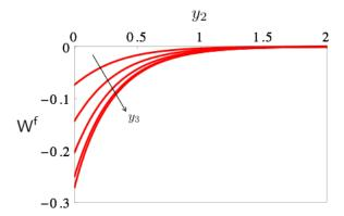
Fig. 3 W<sup>f</sup> is a universal twist boundary layer inducing an out-of-plane displacement near the free side which allows to satisfy zero transverse shear at the boundary. In the graph above, we plot W<sup>f</sup> as a function of  $y_2$  for five values of  $y_3$ ,  $y_3 = 0.1, 0.2, 0.3, 0.4, 0.5$ .
