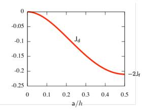
Fig. 9 Graphs of the coefficients  $C_d$  and  $J_d$  as a function of the length a of the crack when  $\nu = 0.25$ . They respectively represent effective rotational and torsional stiffnesses.
