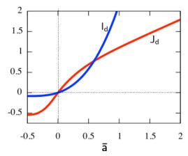
Fig. 6 Graphs of the coefficients  $C_d$ ,  $I_d$  and  $J_d$  as a function of the height  $\bar{a}$  of the defect when  $\nu=0.25$ ,  $\bar{a}>0$  corresponds to a stiffening,  $\bar{a}<0$  to a weakening. While  $I_d$  is a geometric moment, the coefficients  $C_d$  and  $J_d$  can be interpreted as effective rotational and torsional stiffnesses, respectively.
