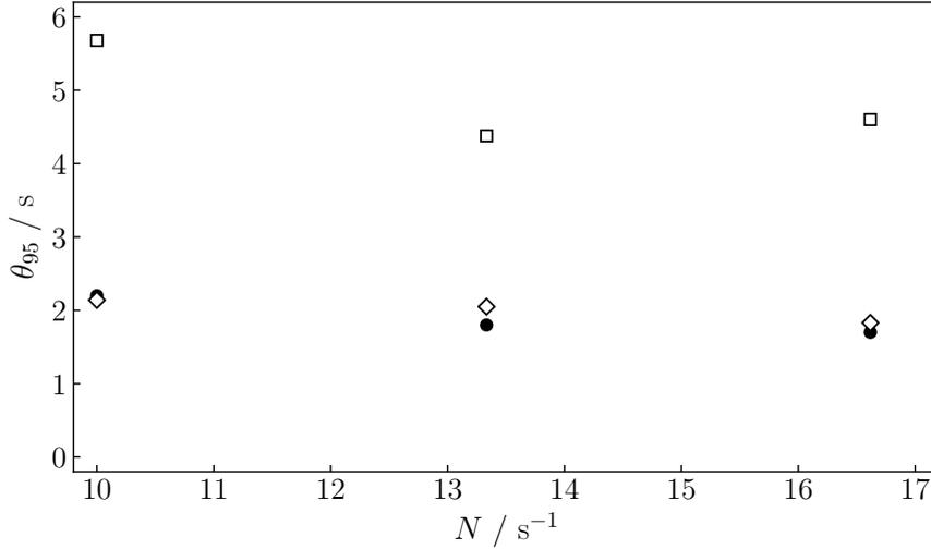
Figure 12: Effect of turbulent Schmidt number on computed mixing time. Comparison with experimental data in  $T_{30}$ . Symbols: experimental (●),  $Sc_t = 0.7$  (□),  $Sc_t = 0.1$  (◇).
