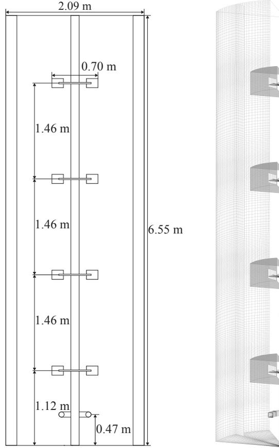
Figure 5: Scheme of the 22 m<sup>3</sup> reactor with four Rushton turbines. On the right, details on the mesh used to model a sixth section of the tank.
