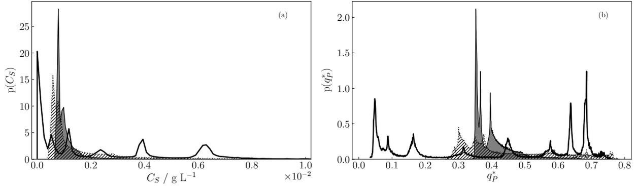
Figure 17: Volumetric distribution of substrate concentration (a) and normalized production rate (b) at  $q_{feed}^I$ ; the y-values are normalized so that the area under each curve is equal to one. The area in gray describes data for 1S, whereas data for 1B and 4R are represented by the hatched and empty areas, respectively.
