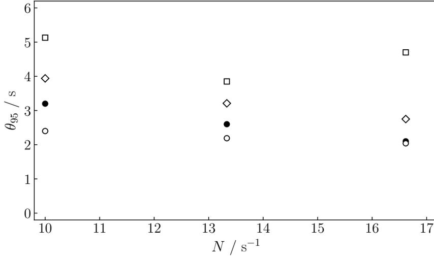
Figure 14: Mixing time in XG 0.25% at different Schmidt numbers. Experimental (●),  $Sc_t = 0.7$  (□),  $Sc_t = 0.2$  (◇),  $Sc_t = 0.1$  (○).
