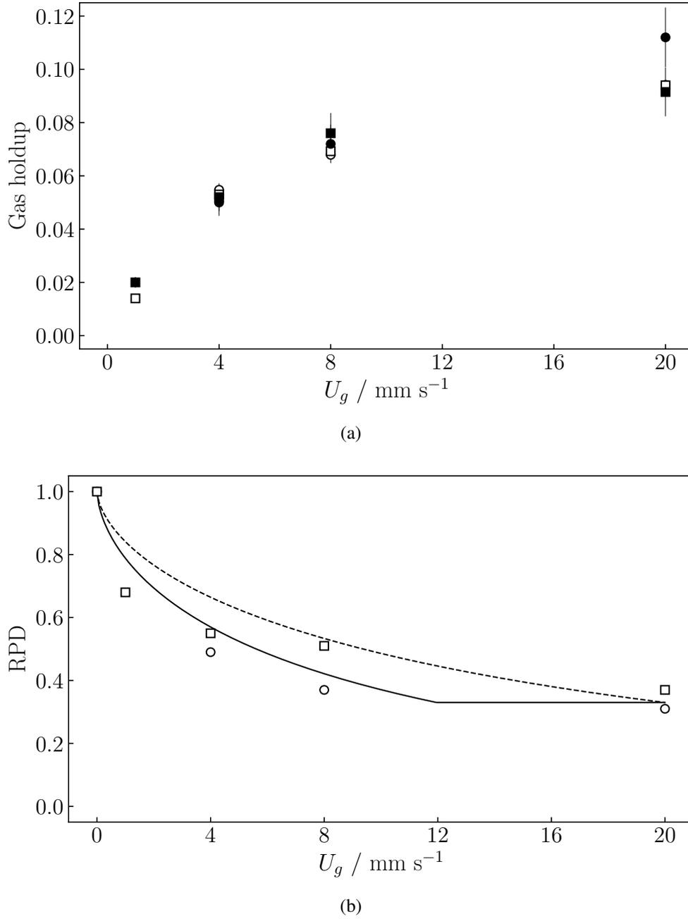
Figure 9: Numerical and measured gas holdup (a) and RPD (b) against superficial gas velocity for two tanks with different diameters.  $T_{30}$ : CFD ( $\circ$ ), experimental ( $\bullet$ ), Eq. (14) (—);  $T_{60}$ : CFD ( $\square$ ), experimental ( $\blacksquare$ ), Eq. (14) (----).
