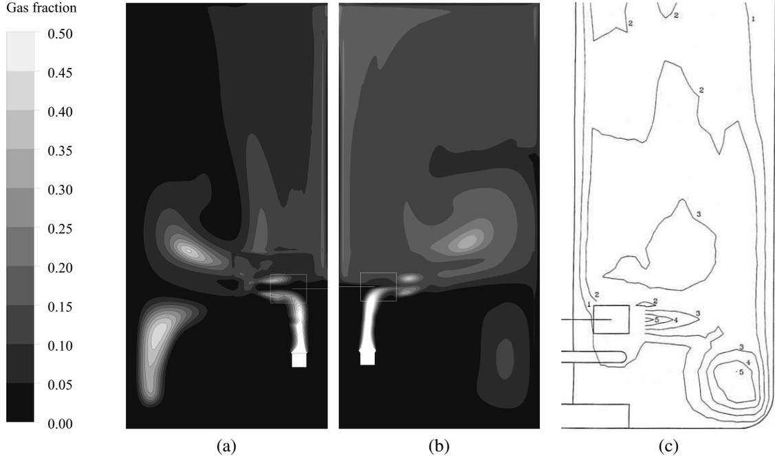
Figure 8: Contours of gas fraction in water in the VC regime based on CFD simulation for  $T_{30}$  (a) and for 1B (b), and measured by [Bombač et al. \(1997\)](#) (c). In order to compare the different cases, the same Froude and Flow numbers were considered.
