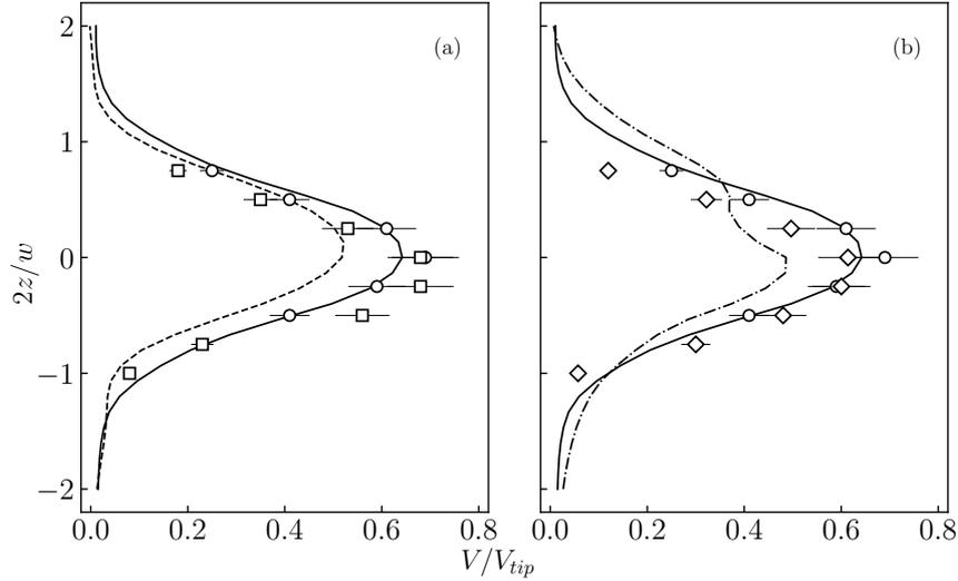
Figure 11: Profile of radial velocity along the blade height ( $w$ ) at the impeller tip in air-water system, for  $N = 5.8 \text{ s}^{-1}$  and  $U_g = 1 \text{ mm s}^{-1}$  (a) and  $U_g = 4 \text{ mm s}^{-1}$  (b). Experimental data:  $U_g = 0$  ( $\circ$ ),  $U_g = 1 \text{ mm s}^{-1}$  ( $\square$ ),  $U_g = 4 \text{ mm s}^{-1}$  ( $\diamond$ ); simulation:  $U_g = 0$  (—),  $U_g = 1 \text{ mm s}^{-1}$  (---),  $U_g = 4 \text{ mm s}^{-1}$  (-.-).
