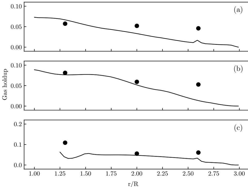
Figure 7: CFD and experimental gas fraction in water at  $N = 8.3 \text{ s}^{-1}$  and  $U_g = 8 \text{ mm s}^{-1}$ ; data were taken in  $T_{60}$  at different heights: impeller height (a), 200 mm (b) and 350 mm above the impeller disk (c). Symbols: CFD (—), experimental (●).
