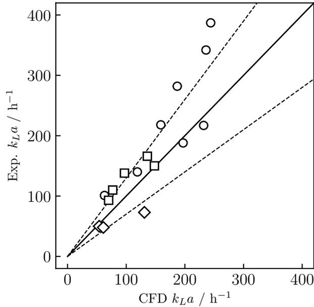
Figure 15: Average volumetric mass transfer coefficient from simulations and experiments. Data are for water ( $\circ$ ), xanthan gum 0.25% ( $\square$ ), and xanthan gum 0.50% ( $\diamond$ ); the dashed lines represent an error  $\pm 30\%$ .
