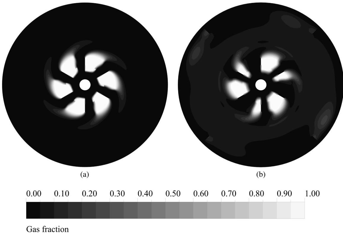
Figure 6: Gas cavity structures at  $U_g = 8 \text{ mm s}^{-1}$  by using MRF (a) and SM models (b). A sixth of the domain was simulated in the case of the MRF approach; to facilitate the comparison, the partial geometry was repeated in post-processing to represent the full tank.
