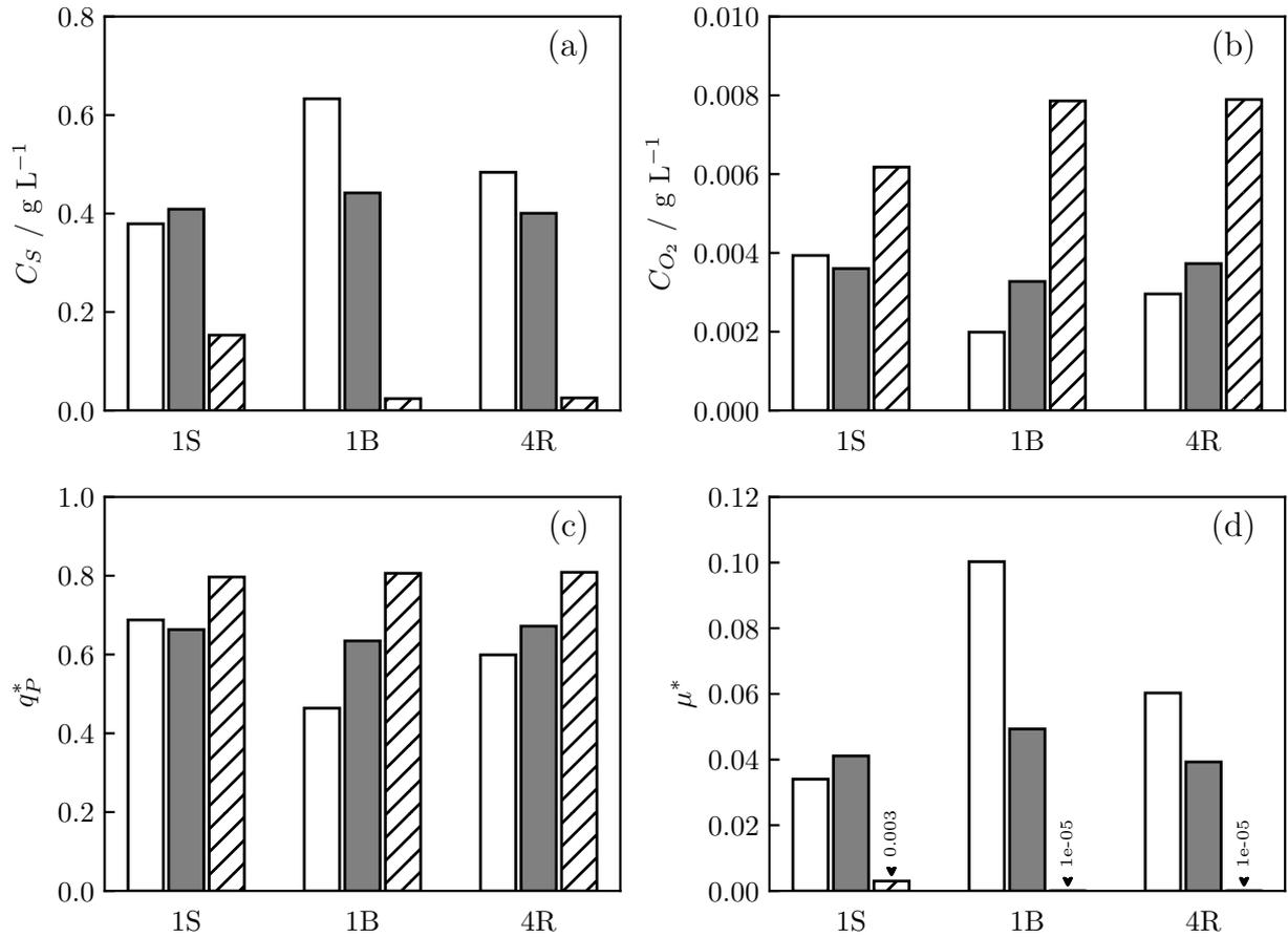
Figure 19: Nutrients concentration (a,b) and normalized production (c) and growth (d) rates for the case  $q_{feed}^{II}$ . CFD and perfect-mixing values are reported in white and gray, respectively. The hatched bars represent estimated values at  $k_L a = 200 \text{ h}^{-1}$ .
