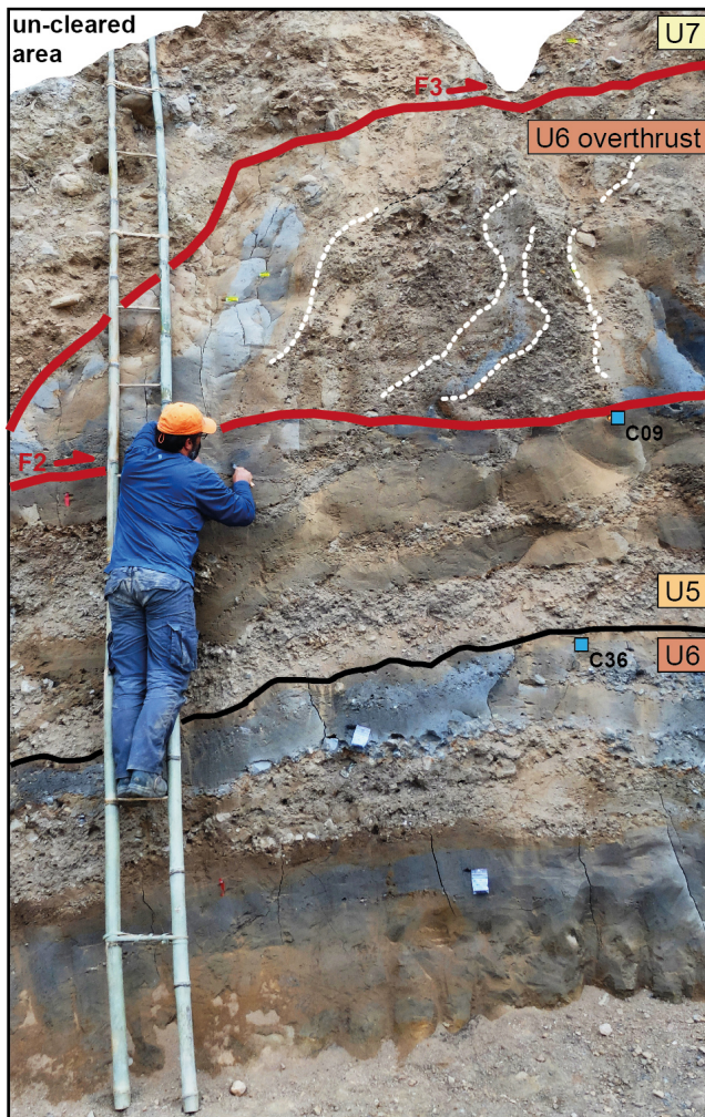
Figure 6. Enlarged photograph of the lower part of the exposure (see Fig. 5a for location) showing (1) sub-horizontal deposits of U5 and U6 below the thrust fault F2 and (2) the overturned limb of U6 and U7 characterized by tilted gravel and silty layers and pebbles, respectively.
