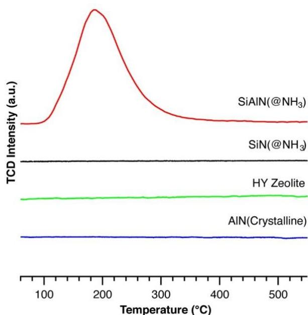
**Fig. S9** Comparison of H<sub>2</sub>-TPD profiles of **PTSiAlN** sample with those of reference samples of **SiN** sample, commercially available crystalline AlN and zeolite samples.
