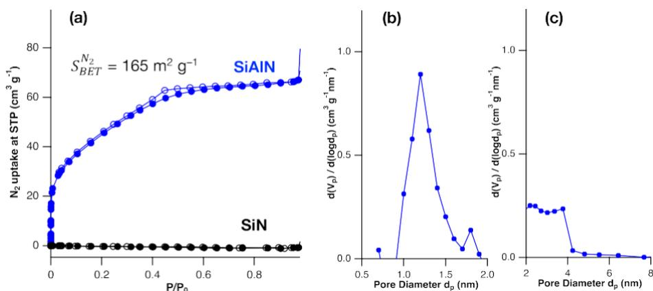
**Fig. S4** (a) N<sub>2</sub> adsorption-desorption isotherms at –196 °C for the polymer-derived amorphous **SiAlN** and **SiN** samples, and pore size distribution curves of the **SiAlN** sample characterized by (b) MP plot and (c) BJH plot.
