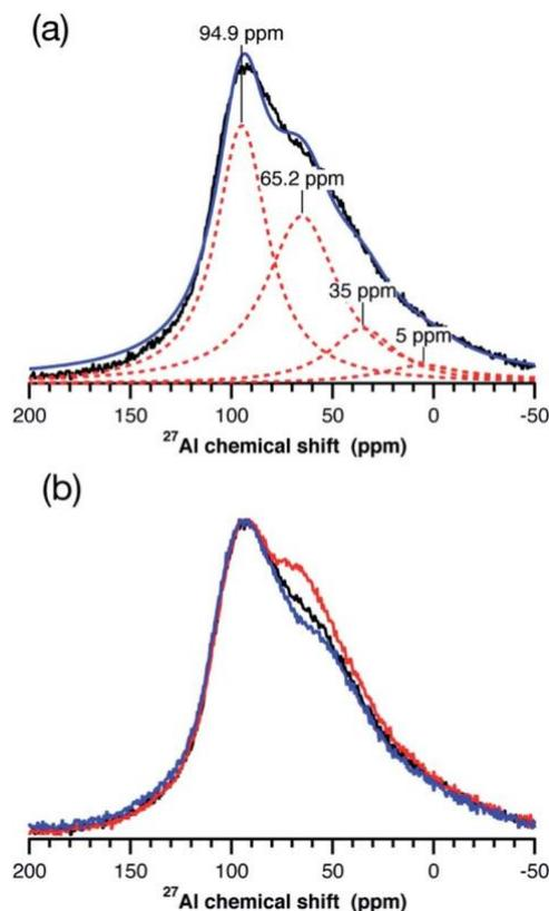
Fig. 7 (a) A typical <sup>27</sup>Al MAS NMR spectrum of the PTSiAlN sample. The black line represents experimental data, the blue line represents curve-fitting results indicated by Lorentzian curves and the red dashed line represents sub-peaks. (b) <sup>27</sup>Al MAS NMR spectra recorded for PTSiAlN
