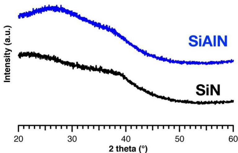
**Fig. S3** Typical XRD patterns of samples after pyrolysis at 1000 °C under flowing NH<sub>3</sub>.
