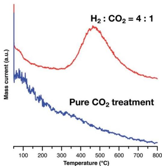
Fig. 9 Post reaction TPD-MS profiles of  $CO_2$  ( $m/z$  44) under an Ar flow. The measurements were performed after exposure to a mixed gas with a 4 : 1 molar ratio of  $H_2$  and  $CO_2$  (Red) and pure  $CO_2$  at  $400\text{ }^\circ\text{C}$  (Blue).
