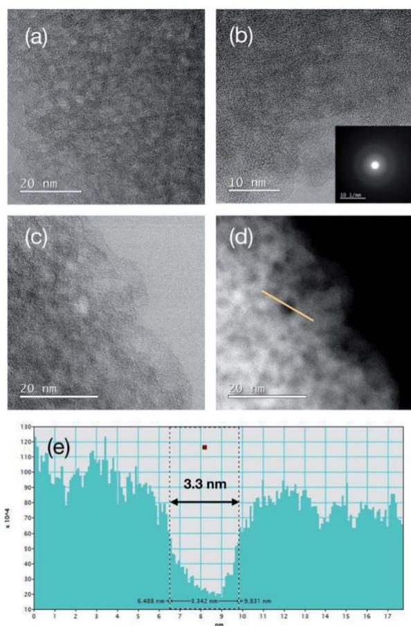
Fig. 1 TEM observation of polymer-derived amorphous SiAlN. (a) HRTEM image, (b) high magnification TEM image and the corresponding SAED pattern obtained, (c) BF-STEM image, (d) HAADF-STEM image and (e) line scanning result for the spot with dark contrast in (d).
