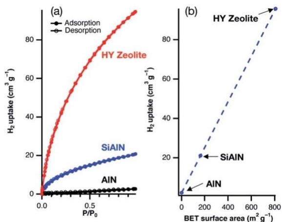
Fig. 5 (a) Volumetric H<sub>2</sub> adsorption and desorption isotherms at  $-193\text{ }^{\circ}\text{C}$  for PTSiAlN and commercially available crystalline AlN and zeolite samples. (b) The correlation between the H<sub>2</sub> uptake and measured BET surface area.
