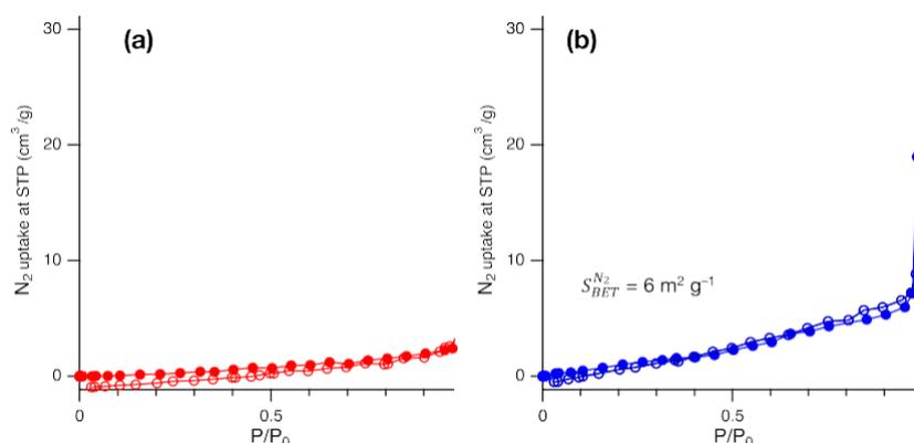
**Fig. S5** Reference data of N<sub>2</sub> adsorption and desorption isotherms at –196 °C. Polymer-derived **SiAlN** pyrolyzed (a) at 1000 °C under N<sub>2</sub> and (b) at 700 °C under NH<sub>3</sub>.
