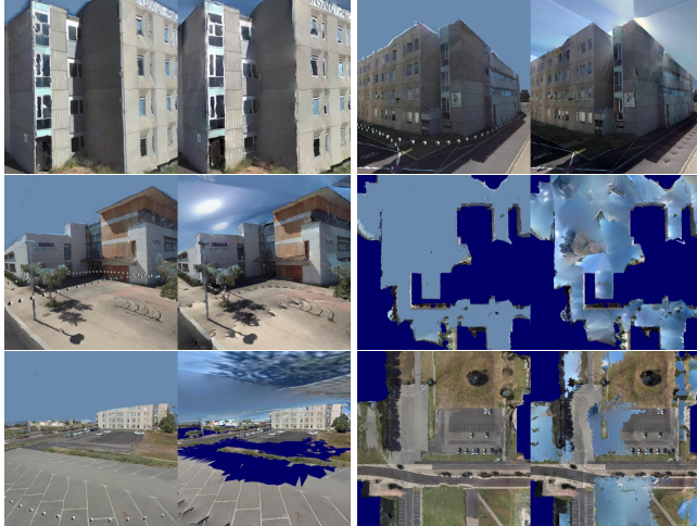
Fig. 9. Comparison between our method (first and third columns) and [16] (second and fourth columns). Our method improves texture near edges (top) and in the sky (middle), it does not remove slanted triangles (bottom).
