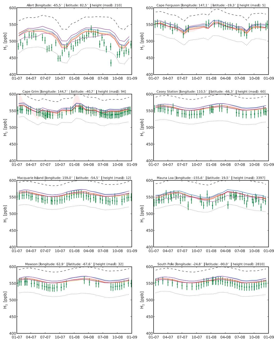
**Figure 2.** Comparison of modeled monthly median H<sub>2</sub> mixing ratios with available measurements from the CSIRO flask sampling network. The circles represent the event samples. The following model scenarios are shown: S1 (dotted), S2 (dashed), S3a (blue), S3b (orange), S3c (red), S4 (magenta), and S5 (purple). The shaded areas indicate the lower and upper quartiles of the variability in the model results for scenario S3c (red). Dates on the x axis are shown in MM-YY format.
